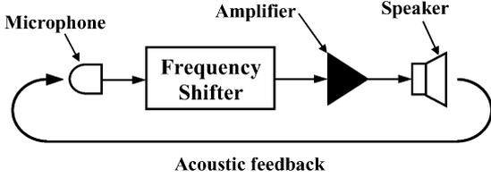
Fig. 4. Frequency shifter is inserted to suppress oscillation due to acoustic feedback.
