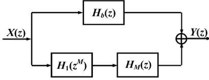
Fig. 2. Structure for the synthesis of a Hilbert transformer using the FRM technique.
