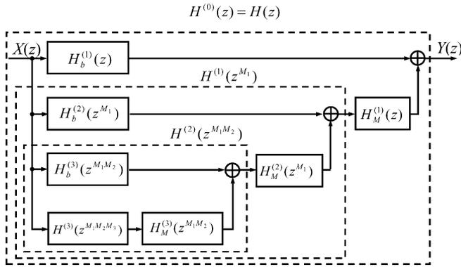
Fig. 7. Three-level masking structure.
