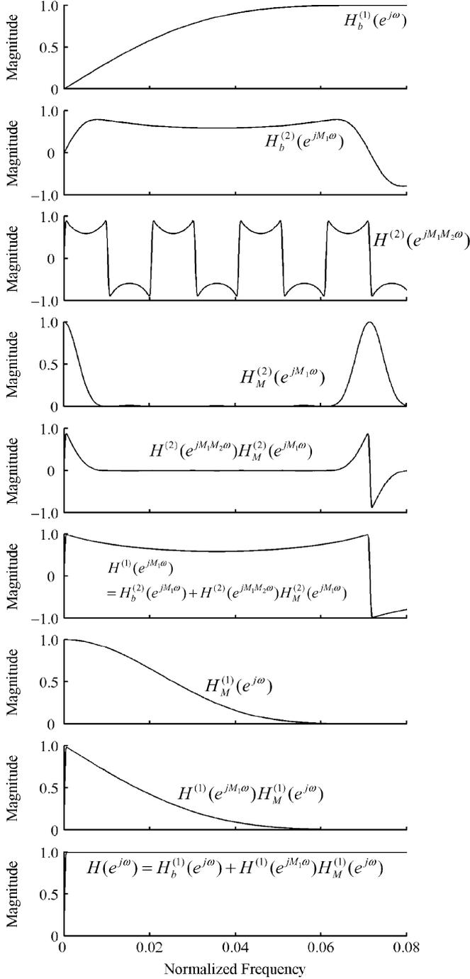
Fig. 9. Frequency responses of the individual subfilters and the overall filter.
