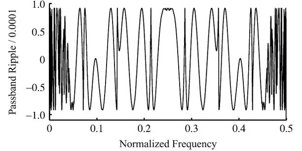
Fig. 8. Passband ripples of the Hilbert transformer. The frequency axis is normalized against the sampling frequency.
