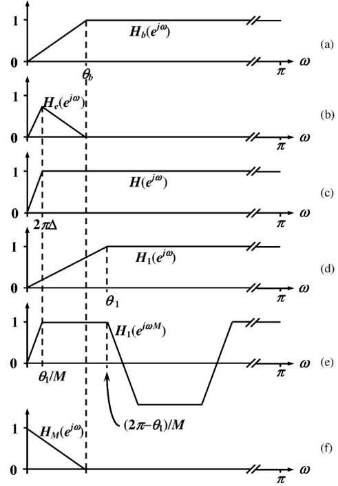
Fig. 3. Frequency responses of the subfilters for even length  $H_b(z)$ . Note that  $\theta_1/M = 2\pi\Delta$ .  $2\pi\Delta$  is the transition width of the desired transfer function.
