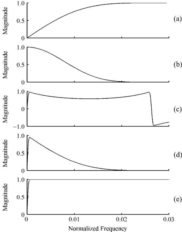
Fig. 6. Frequency responses of the individual subfilters. (a)  $H_b(e^{j\omega})$ , (b)  $H_M(e^{j\omega})$ , (c)  $H_1(e^{jM\omega})$ , (d)  $H_M(e^{j\omega})H_1(e^{jM\omega})$ , (e)  $H_b(e^{j\omega}) + H_M(e^{j\omega})H_1(e^{jM\omega})$ .
