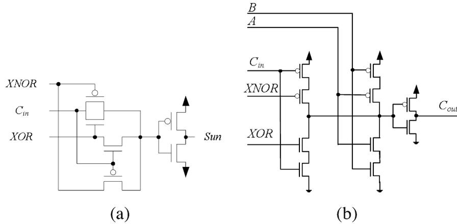
Fig. 5. (a) Module 2 and (b) Module 3.
