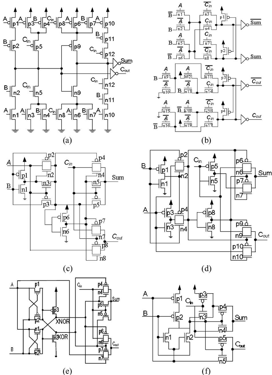
Fig. 1. Full adder cells of different logic styles. (a) C-CMOS. (b) CPL. (c) TFA. (d) TGA. (e) 14 T. (f) 10 T.
