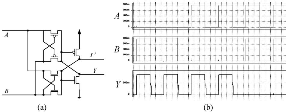
Fig. 3. XOR-XNOR 6 T gate and its worst-case delay waveform.
