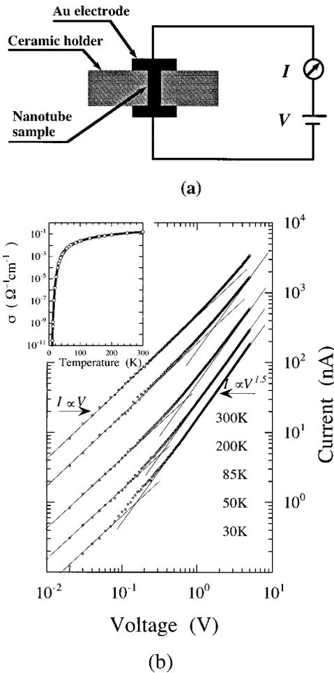
FIG. 4. (a) Schematic diagram illustrating the experimental setup for electrical measurements for the SWCNs, and (b) the experimental dc  $I-V$  curves (open circles) at different temperatures plotted on a log-log scale. The fittings are shown as solid lines with  $I \propto V$  in the low bias region and  $I \propto V^{3/2}$  in the high bias region. The inset of (b) shows the conductivity measured near zero bias as a function of temperature.
