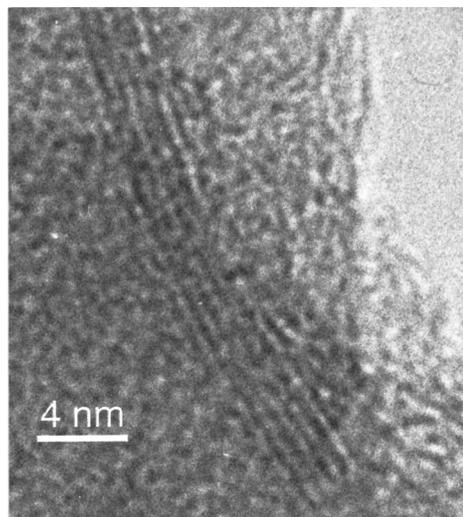
FIG. 1. Transmission electron microscope (TEM) image shows the SWCNs which are slightly bent. The TEM image was taken after the AFI framework was removed using HCl acid, and the SWCNs were exposed in free space.
