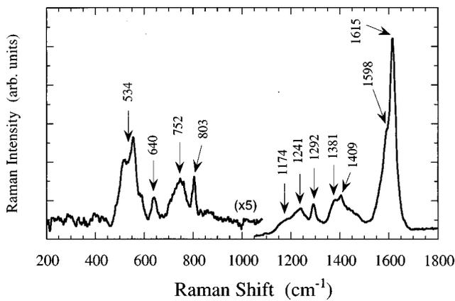
FIG. 2. Raman spectrum of the SWCNs measured at room temperature using the 632.8 nm line of a He-Ne laser as the excitation.
