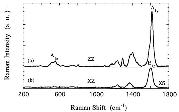
FIG. 3. Polarized Raman spectra of the SWCNs measured in (a) ZZ configurations, and (b) XZ configuration. In the ZZ configuration, the polarizations of the incident and the scattered lights are parallel to each other and are polarized along the nanotube direction; in the XZ configuration the polarizations of the incident and the scattered lights are perpendicular to each other.
