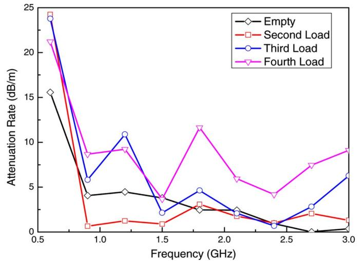
Fig. 4. Attenuation rate as a function of frequency for the closed scaled model.
