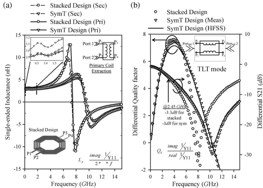
Fig. 3. (a) Individual coil inductance plot of the stacked and the proposed transformer designs together with the 3-D and the cross-sectional view of the stacked design. (b) Differential  $Q$  and  $S_{d21}$  plots of the stacked and the proposed transformer designs.
