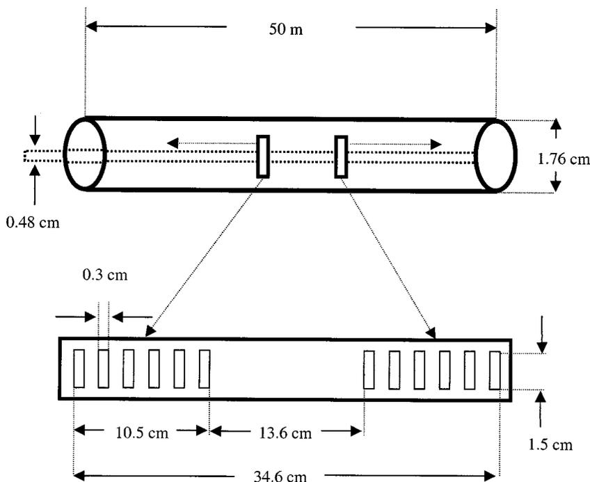
Fig. 1. The configuration of the radiated-mode leaky feeder.
