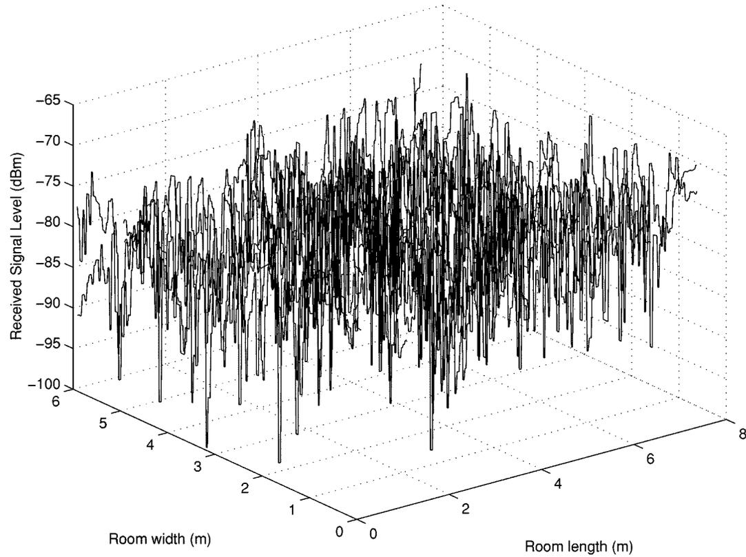
Fig. 4. The received signal levels in the room.
