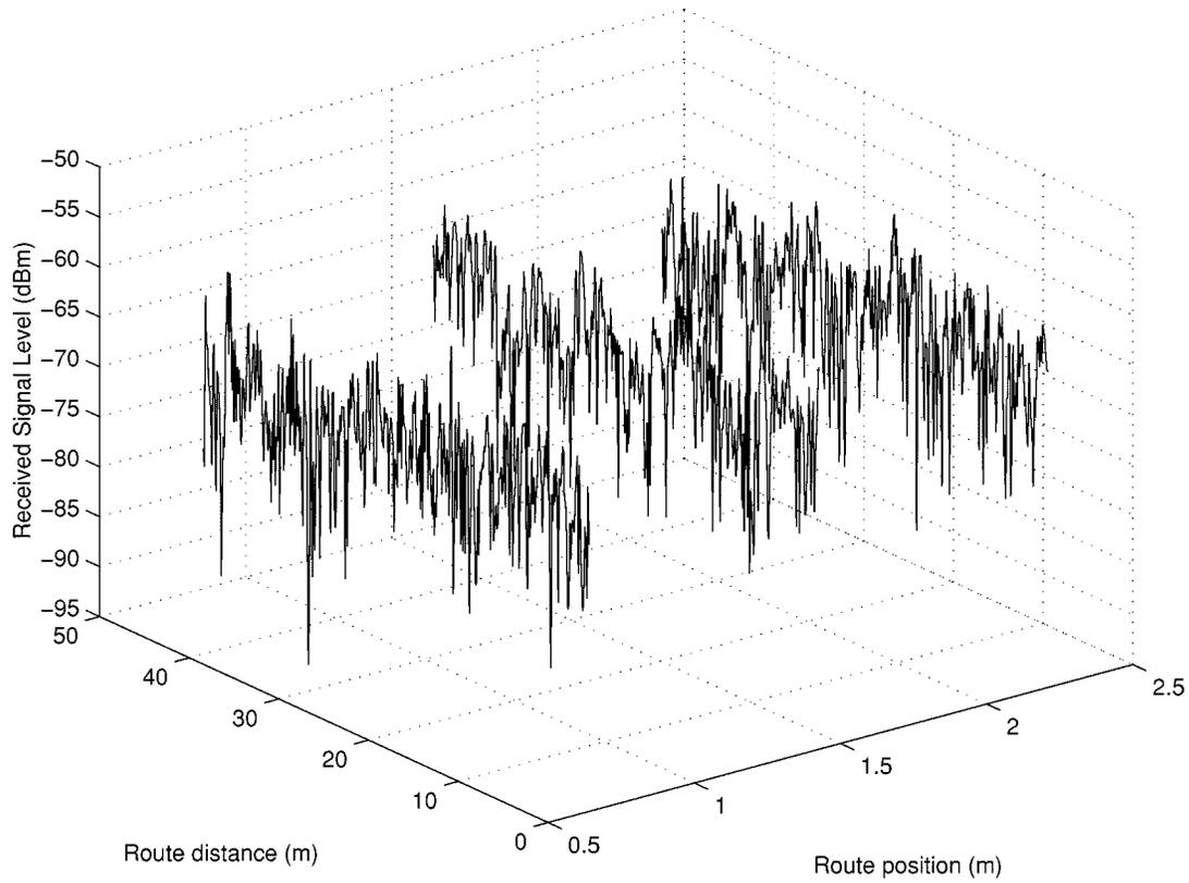
Fig. 3. The received signal levels in the corridor.
