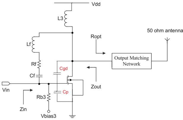
Figure 2. Output stage with an LRC stabilizer.
