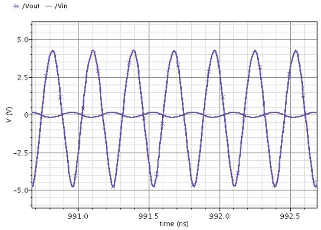
Figure 8. Input and output voltage @  $P_{1dB}$ .
