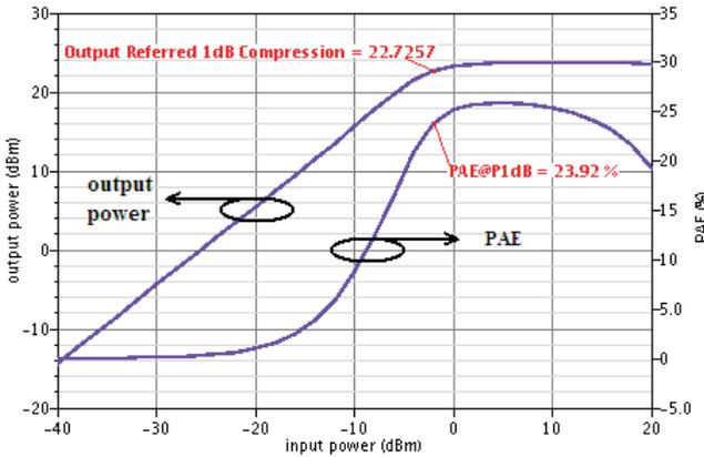
Figure 7. Output power and PAE VS input power.
