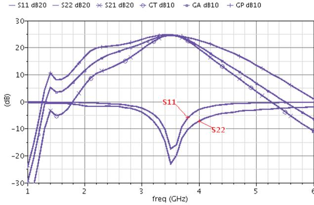
Figure 6. Results for small signal S-parameter simulation.
