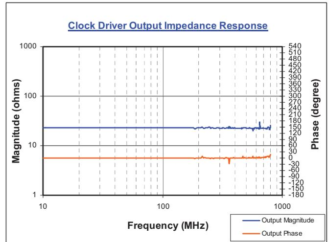
Figure 8. Measured Clock Driver Output Impedance Characteristic
