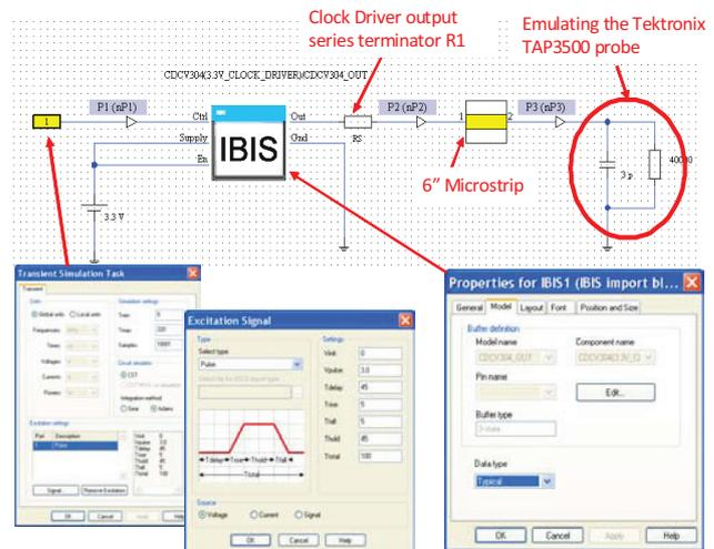
Figure 9. CST-DS IBIS Transient Simulation Setup
