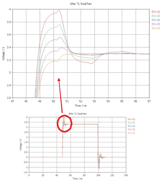
Figure 10. IBIS Simulation Using Parameter Sweep to Determine the Series Resistance R1
