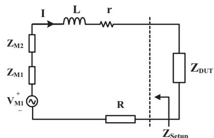
Figure 2. Simplified Equivalent Circuit of the Two-Probe Setup
