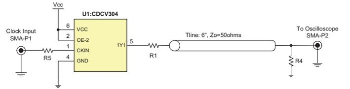
Figure 3. Test circuit Schematic for two Probe Measurement
