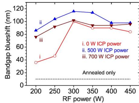
FIG. 3. (Color online) Band-gap blueshift vs rf power under (i) 0 W ICP power, (ii) 500 W ICP power, and (iii) 700 W ICP power. The plasma exposure time was fixed at 30 s.
