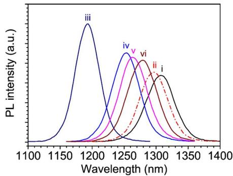
FIG. 4. (Color online) PL spectra measured at 77 K from (i) an as-grown sample, (ii) a sample exposed to argon plasma and annealed with a 300-nm-thick  $\text{SiO}_2$  layer ( $\text{SiO}_2$  layer was removed before PL measurement), and bare samples exposed to argon plasma, chemically wet etched in  $\text{HCl}:\text{H}_2\text{O}$  (1:2) solution for (iii) 0 min, (iv) 3 min, (v) 5 min, and (vi) 7 min, and finally annealed.
