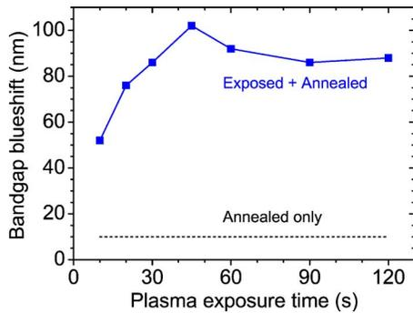
FIG. 1. (Color online) Band-gap blueshift vs Ar plasma exposure time for samples being exposed and annealed. The level of thermal shift is obtained from an annealed-only sample.
