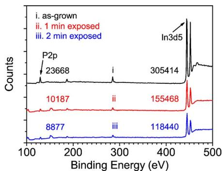
FIG. 2. (Color online) XPS spectra measured from the InP cap layer for (i) as-grown sample and samples exposed to Ar plasma for (ii) 1 min and (iii) 2 min. The counts from In  $3d5$  and P  $2p$  core levels for the three samples are labeled as well.
