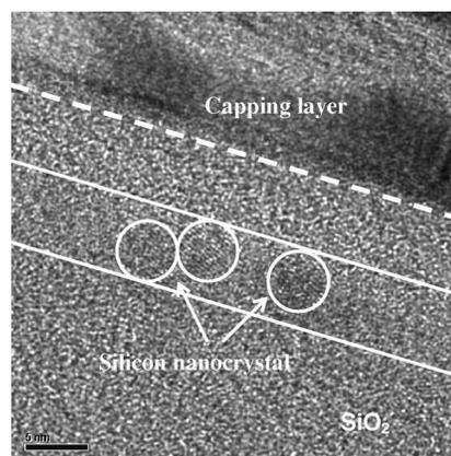
FIG. 1. Cross-sectional high-resolution TEM image of sample 2.
