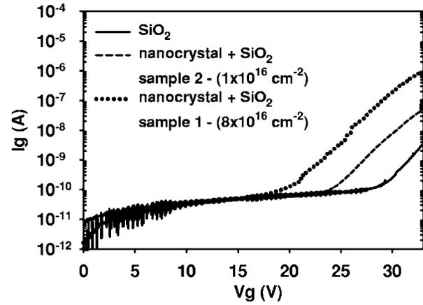
FIG. 3. Current-voltage characteristics of sample 1, sample 2, and the pure  $\text{SiO}_2$  sample.
