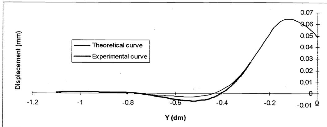
Fig. 8 Typical experimental and theoretical deflection curves of a Type 3 structure
