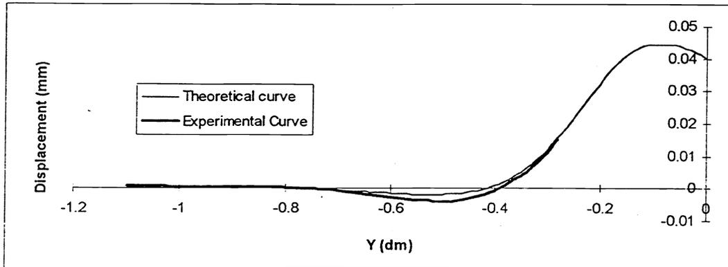
Fig. 7 Typical experimental and theoretical deflection curves of a Type 2 structure
