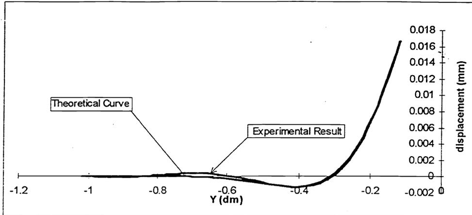
Fig. 6 Typical experimental and theoretical deflection curves of a Type 1 structure
