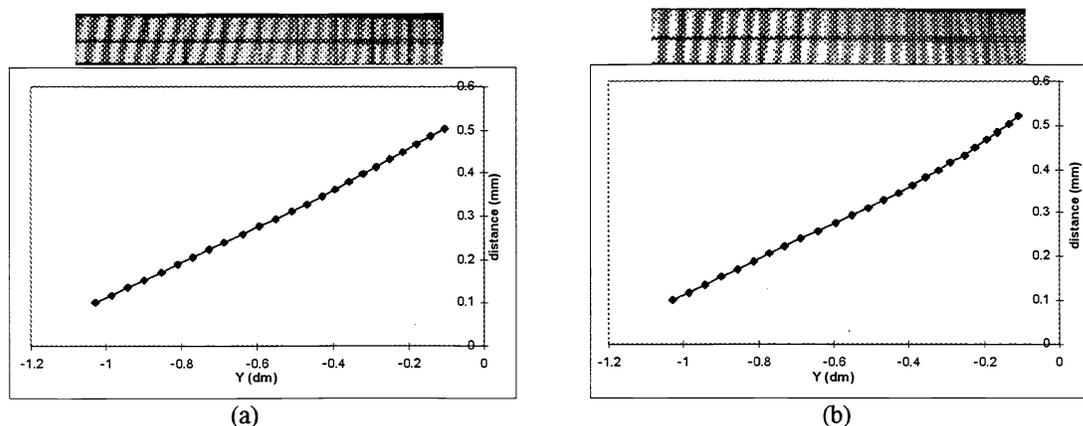
Fig. 5 Typical Moiré patterns and surface contours of a Type 1 structure
