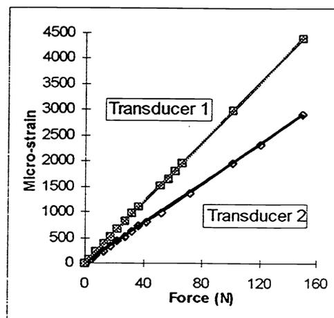
Fig. 3 Calibration charts of the force transducers used, Transducer 1 being located at point  $O_1$ , and Transducer 2 being located at point  $O_2$
