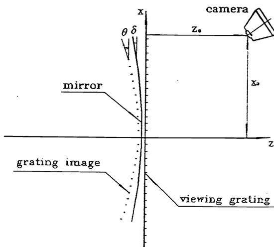
Fig. 2 Schematic layout of the mirror-image method
