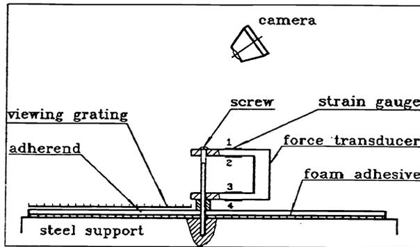
Fig. 1 General arrangement for testing the stiffness of the adhesive layer of a specimen
