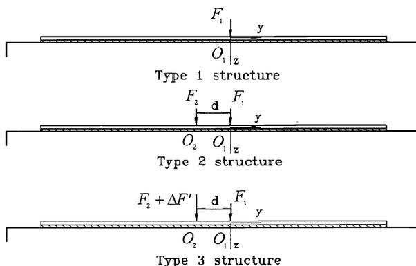
Fig. 4 Methods of loading the test specimens
