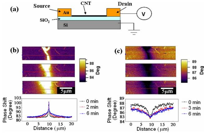
FIG. 2. (Color online) (a) Experimental setup with dc bias applied to the drain, the gate grounded and the source floating,  $V_{\text{tip}}=3$  V during the interleave scan, and charging images and cross section profiles when (b)  $V_{\text{drain}}=-5$  V and (c)  $V_{\text{drain}}=+5$  V.
