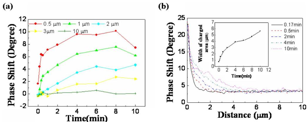
FIG. 3. (Color online) (a) Phase shift as a function of time at different distances away from the SWNT for  $V_{\text{drain}}=-5$  V, showing the accumulation of charges over time. (b) Phase shift as a function of distance from the SWNT. Inset of (b) shows the extension of the charged area as a function of time.
