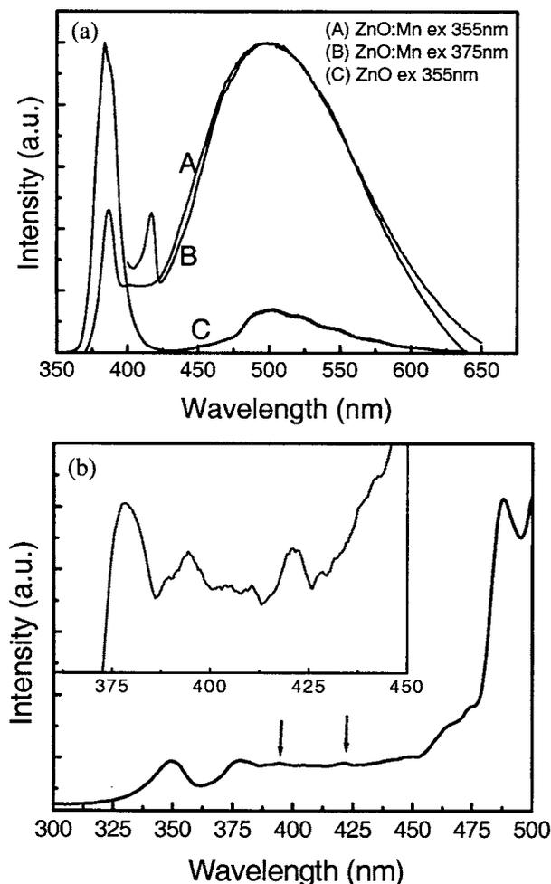
FIG. 5. PL (a) and PLE (b) spectra of ZnO:Mn tetrapodes. The curves A, B, and C in (a) correspond to ZnO:Mn, ZnO:Mn, and ZnO samples excited by 355 nm (A), 375 nm (B), and 355 nm (C), respectively. The insert in (b) shows the two enlarged peaks indicated by the arrows.
