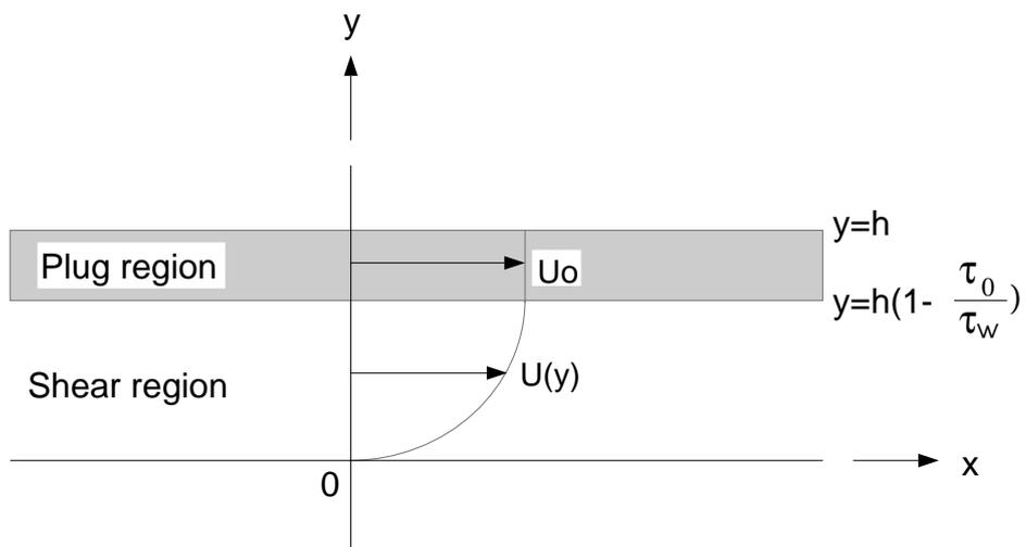
Figure 1: Velocity profile for Bingham fluid over a horizontal plate
