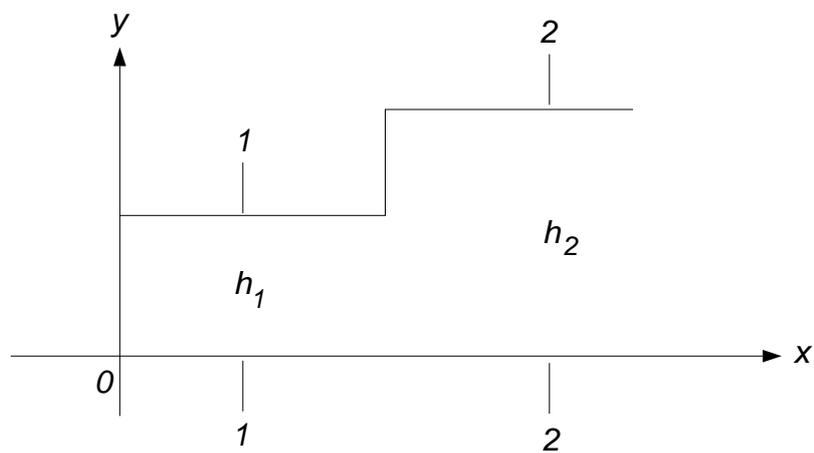
Figure 2: Sketch for a hydraulic jump
