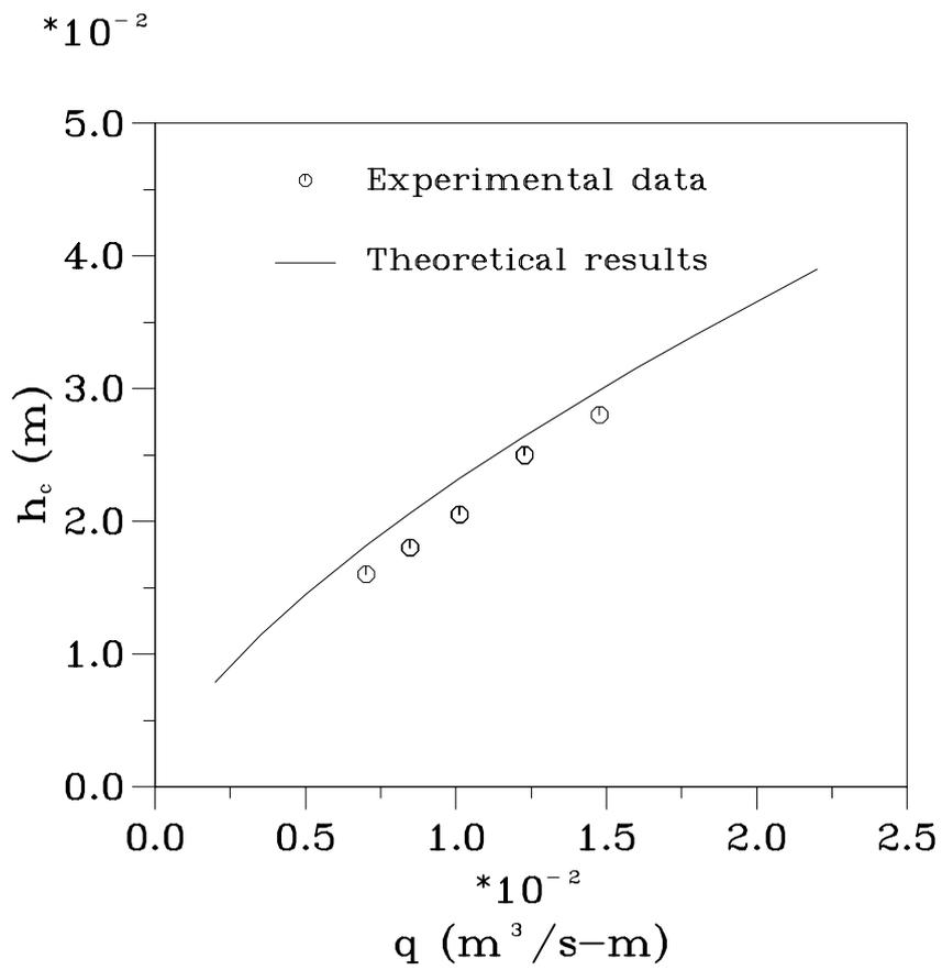
Figure 9: Comparison of the critical depth
