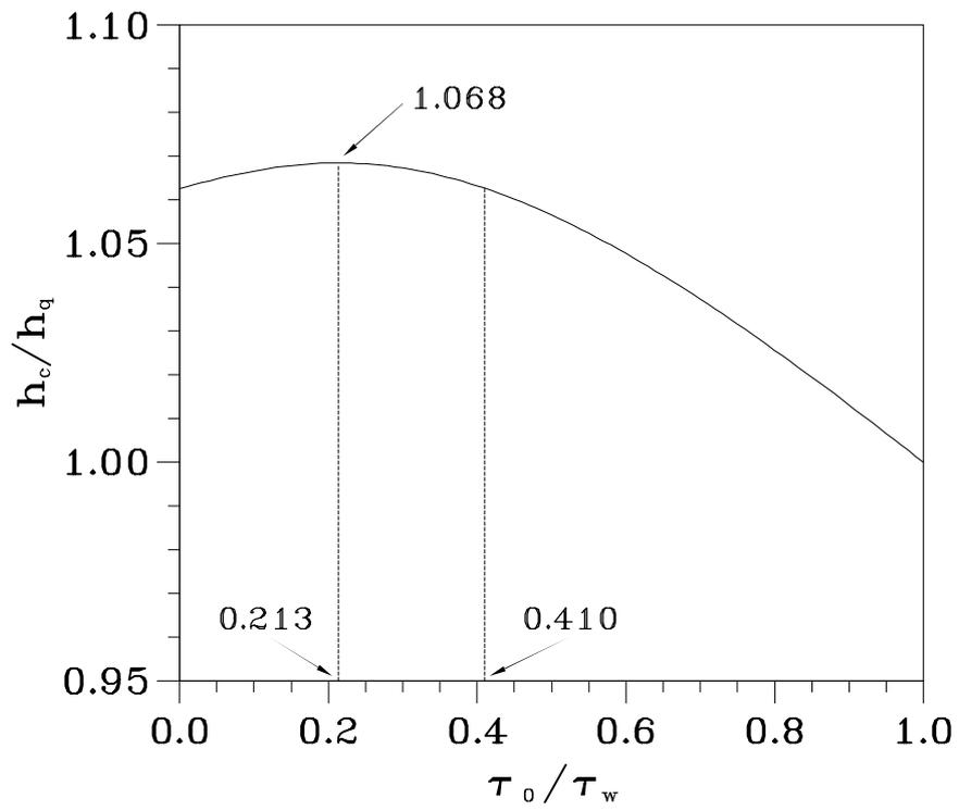
Figure 3: Critical depth versus dimensionless yield stress  $\tau_0/\tau_w$
