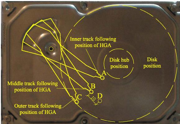
Fig. 2. Locations of four holes (marked from A to D) drilled on the HDD top cover for the pressure fluctuation measurements. Three HGA working positions in inner, middle and outer track following are indicated respectively. The unit in the figure is mm.
