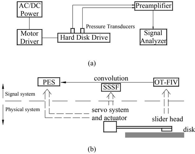
Fig. 1. Schematic illustration of the experimental setup. (a) The experimental setup for the pressure fluctuation measurement, where a 3.5-inch Seagate hard disk drive with one disk and two HGAs is driven by a motor driver at a speed of 7200 rpm, and (b) the time domain signal transmission from the slider OT-FIV to the positioning error signal (PES) via convolution with the servo sensitivity function (SSSF) in an HDD.
