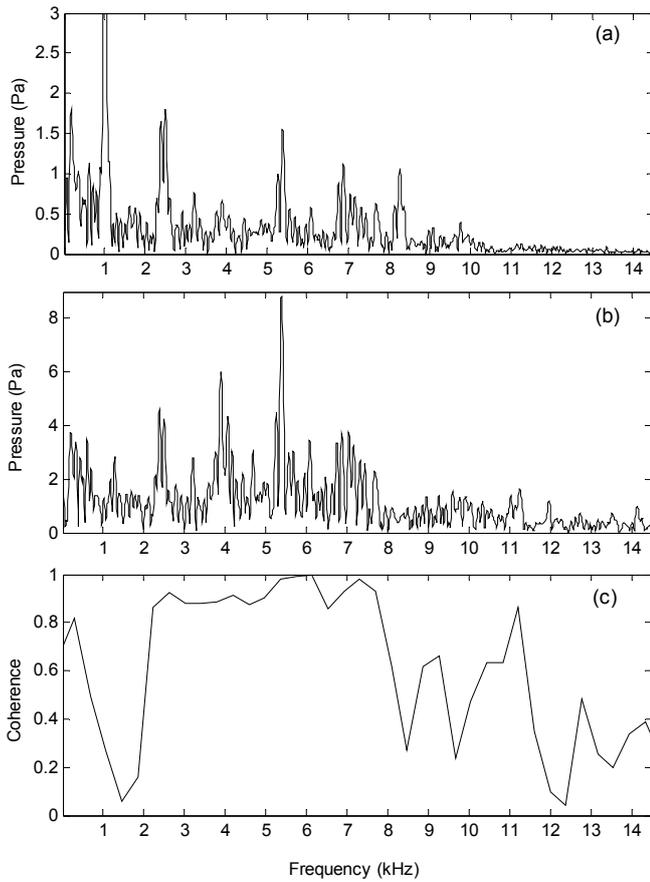
Fig. 8. (a) Calculated spectra of pressure fluctuation at the point  $P_3$  indicated in Fig. 7, (b) calculated spectra of drag pressure  $P_d$  on the HGA that is from subtracting the collected transient pressure at point  $P_2$  from that at  $P_1$  in Fig. 7, and (c) spatial coherence between the drag pressure  $P_d$  and the pressure fluctuation at the point  $P_3$ .
