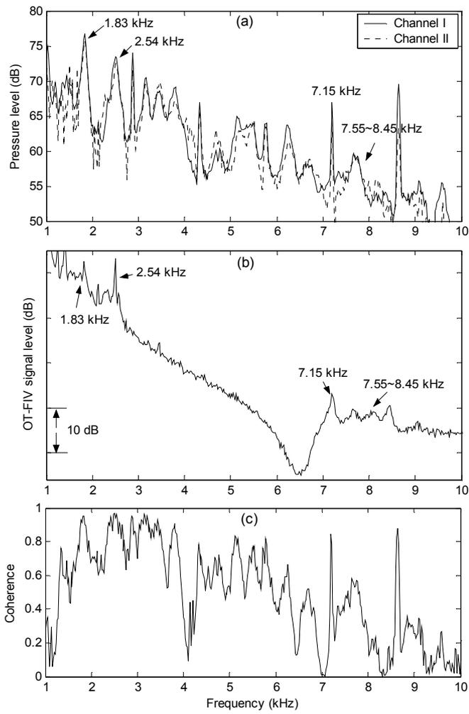
Fig. 5. The HGA heads are in the middle track following position (a) Spectra of measured pressure fluctuation level from two channels (Channel I and Channel II), (b) the spectra of the off-track flow-induced vibration (OT-FIV) of the slider and (c) measured spatial coherence between two channels of pressure fluctuation, where Channel I and II transducers are placed on the hole B and D respectively.
