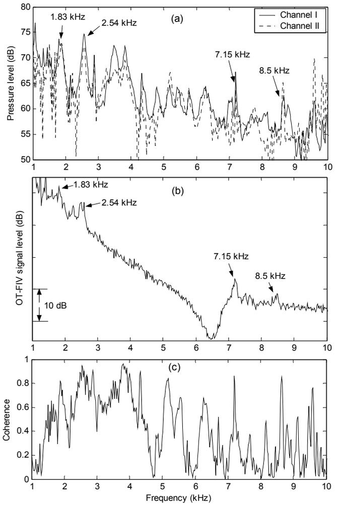
Fig. 4. The HGA heads are in the inner track following position. (a) Spectra of measured pressure fluctuation level from two channels (Channel I and Channel II), (b) spectra of the off-track flow-induced vibration (OT-FIV) of the slider and (c) measured spatial coherence between two channels of pressure fluctuation, where Channel I and II transducers are placed on the hole A and B respectively.
