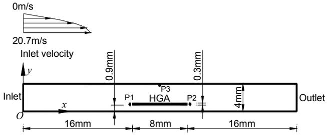
Fig. 7. Geometry of two-dimensional channel flow around a rectangular block to simplify the large eddy simulation on turbulent airflow around the HGA in the middle track following mode. The HGA is simplified as a rectangular block in the flow and dimensions are in accord with those inside the actual HDD in experiments.
