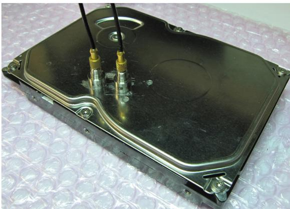
Fig. 3. The photograph of the HDD with two pressure transducers mounted on two selected holes on the cover, while the other two holes are sealed with adhesive tape.
