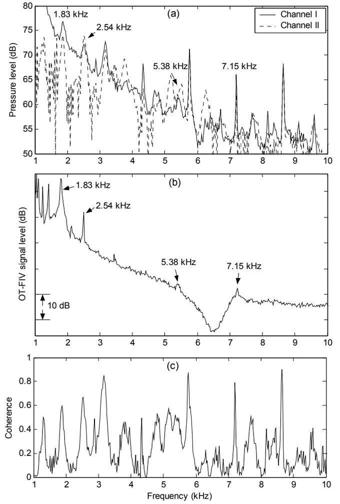
Fig. 6. The HGA heads are in the outer track following position. (a) Spectra of measured pressure fluctuation level from two channels (Channel I and Channel II), (b) the spectra of the off-track flow-induced vibration (OT-FIV) of the slider and (c) measured spatial coherence between two channels of pressure fluctuation, where Channel I and II transducers are placed on the hole C and B respectively.
