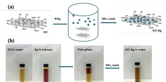
**Scheme 1** Steps for the synthesis of the GO-Ag composites: (a) Schematic presentation of the two-phase synthesis of GO-Ag composites; (b) Photographs of the two-phase synthesis of GO-Ag composites.
