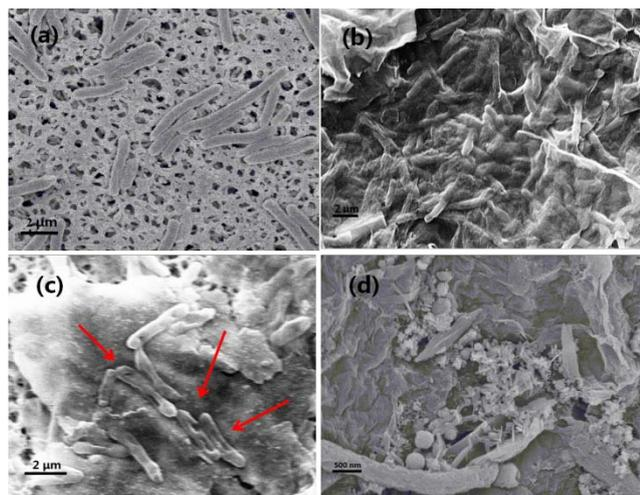
**Fig.6** SEM images of *E. coli* after membrane filtration with different concentration of GO-Ag composites: (a) 0  $\mu\text{g/mL}$ , (b) 20  $\mu\text{g/mL}$ , (c) 50  $\mu\text{g/mL}$ , (d) 100  $\mu\text{g/mL}$ .
