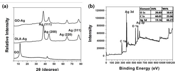
**Fig. 2** (a) XRD patterns of GO sheets, oleylamine-capped Ag nanoparticles and GO-Ag composites. (b) XPS spectra of GO-Ag composites (Inset table is the element weight percentage).
