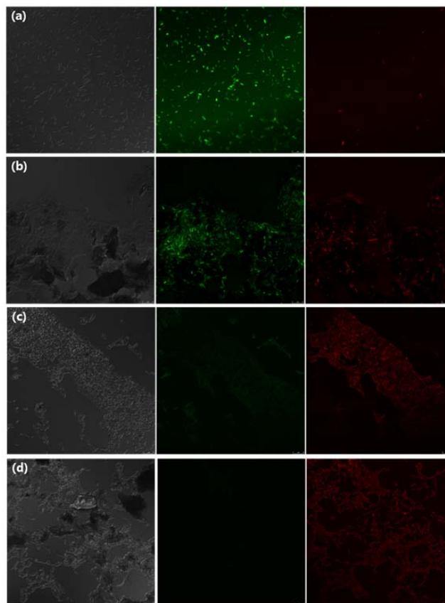
Fig. 5 Real microscopic images and fluorescence microscopic images of bacteria after incubation with different samples in saline solution for 2 h: (a) *E.coli* without samples; (b) *E.coli* with 100 µg/mL of GO sheets; (c) *E.coli* with 100 µg/mL of Ag nanoparticles; (d) *E.coli* with 100 µg/mL of GO-Ag composites.
