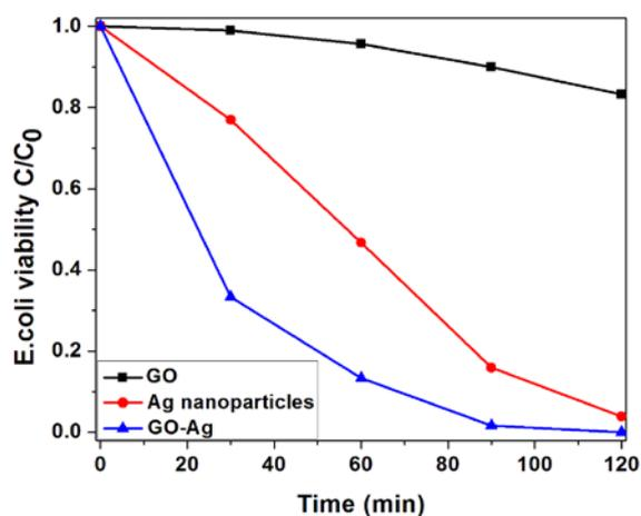
Fig.4 Time course for antibacterial activity of 100 µg/mL of GO sheets, Ag nanoparticles and GO-Ag composites, with an initial *E.coli* concentration of  $3 \times 10^7$  cfu/mL
