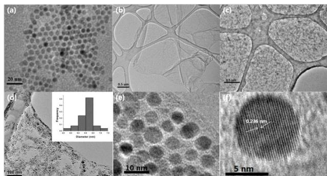
**Fig. 1** TEM images of Ag nanoparticles (a), GO sheets (b), GO-Ag composites (c), (d), (e) and (f). Inset of (d) is the size distribution of Ag nanoparticles on GO sheets.
