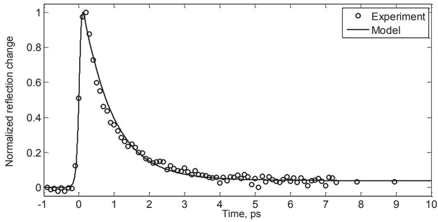
**Fig. 4** Decay kinetics of the reflection change at 632 nm from 300  $\mu\text{m}$  gold plated quartz substrate after the excitation with 350 nm 65 fs laser pulse and theoretical curves for penetration depth  $\kappa=3.0$  nm corresponding to electron-phonon relaxation time equals 0.9 ps.
