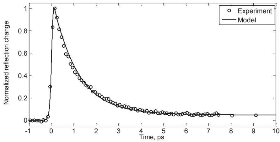
**Fig. 3** Decay kinetics of the reflection change at 590 nm from 300  $\mu\text{m}$  gold plated quartz substrate after the excitation with 350 nm 65 fs laser pulse and theoretical curves for penetration depth  $\kappa=3.8$  nm corresponding to electron-phonon relaxation time equals 1.15 ps.
