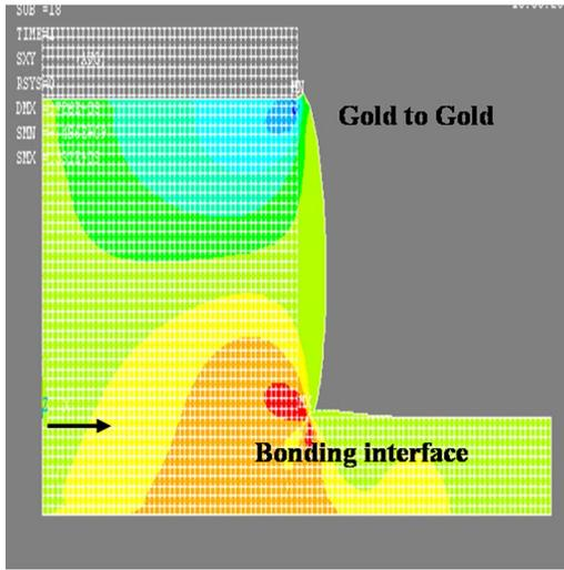
FIG. 7. (Color online) Typical stress contour (undeformed and deformed) diagram illustrating the shear stress distribution for gold bump-10 μm gold model.
