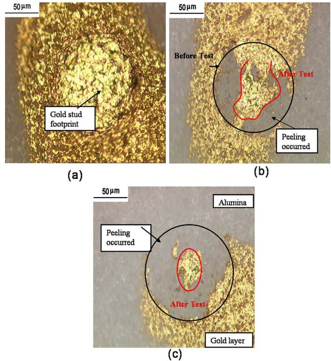
FIG. 9. (Color online) Optical fractographs of Au stud left on alumina substrate at different tool temperatures: (a) 150 °C, (b) 180 °C, and (c) 250 °C.
