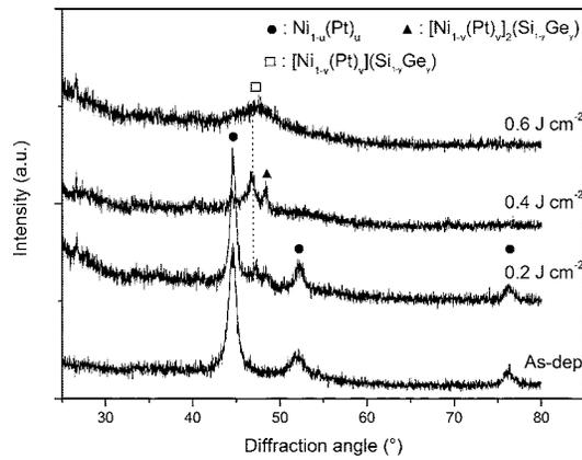
FIG. 1. XRD spectra of the  $\text{Ni}_{1-u}\text{Pt}_u/\text{Si}_{1-x}\text{Ge}_x$  samples after 20-pulsed LTA process. The as-deposited sample has a composition of approximately 96.8 at. % Ni and 3.2 at. % Pt, which is symbolized as  $1-u$  and  $u$  for simplicity. The initial Ge concentration in the  $\text{Si}_{1-x}\text{Ge}_x$  layer was 15%. The  $y$  and  $v$  values in the germanosilicide phases formed are  $<0.15$  and  $\leq 0.032$ , respectively.
