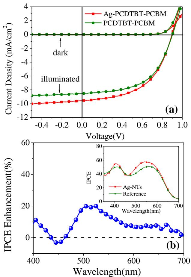
Fig5. (a) J-V characteristics of PCDTBT:PCBM BHJ OPV device with/ without Ag-NTs (b) The percentage enhancement in the IPCE of the devices with Ag-NTs over the reference (without Ag-NTs). Inset shows the IPCE of the two devices.
