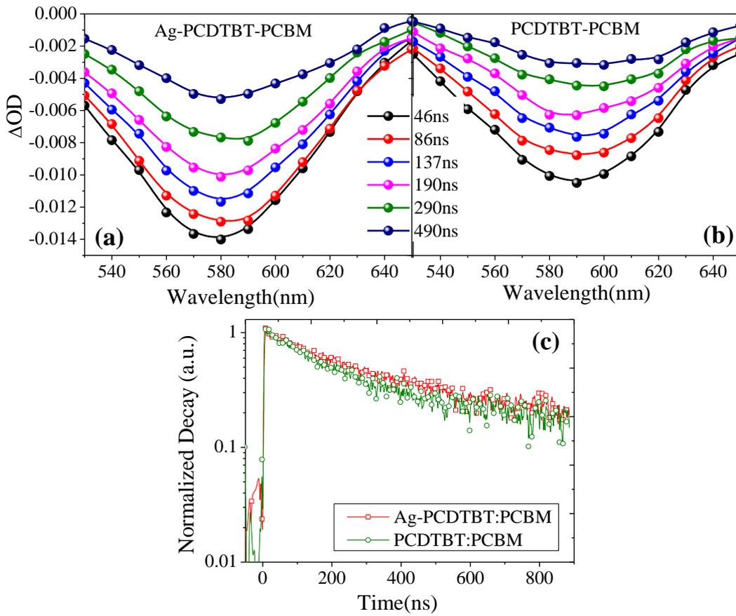
Fig4. ns-TAS spectra of PCDTBT:PCBM bulk-heterojunction films (a) with and (b) without Ag-NTs on a glass substrate. (c) The normalized decay of the two samples at 580nm, showing near invariance of the transient decay dynamics for the samples with and without Ag-NTs.
