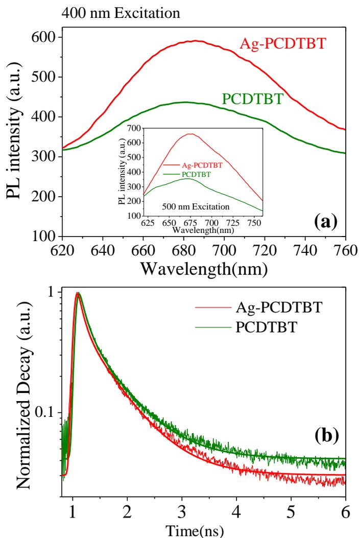
Fig3. (a) Steady-state PL of PCDTBT on glass substrate with/without Ag-NTs excited at (a) 400nm. Inset shows the PL of PCDTBT with/without Ag-NTs excited at 500nm. (b) Time-resolved photoluminescence of PCDTBT on glass substrate with/without Ag-NTs excited at 400nm at a fluence of  $1.5 \mu\text{J}/\text{cm}^2$ . Similar decay transients were obtained for 500 nm excitation. Note that a layer of PEDOT:PSS was spincoated over the substrate or the Ag-NTs in all these samples.
