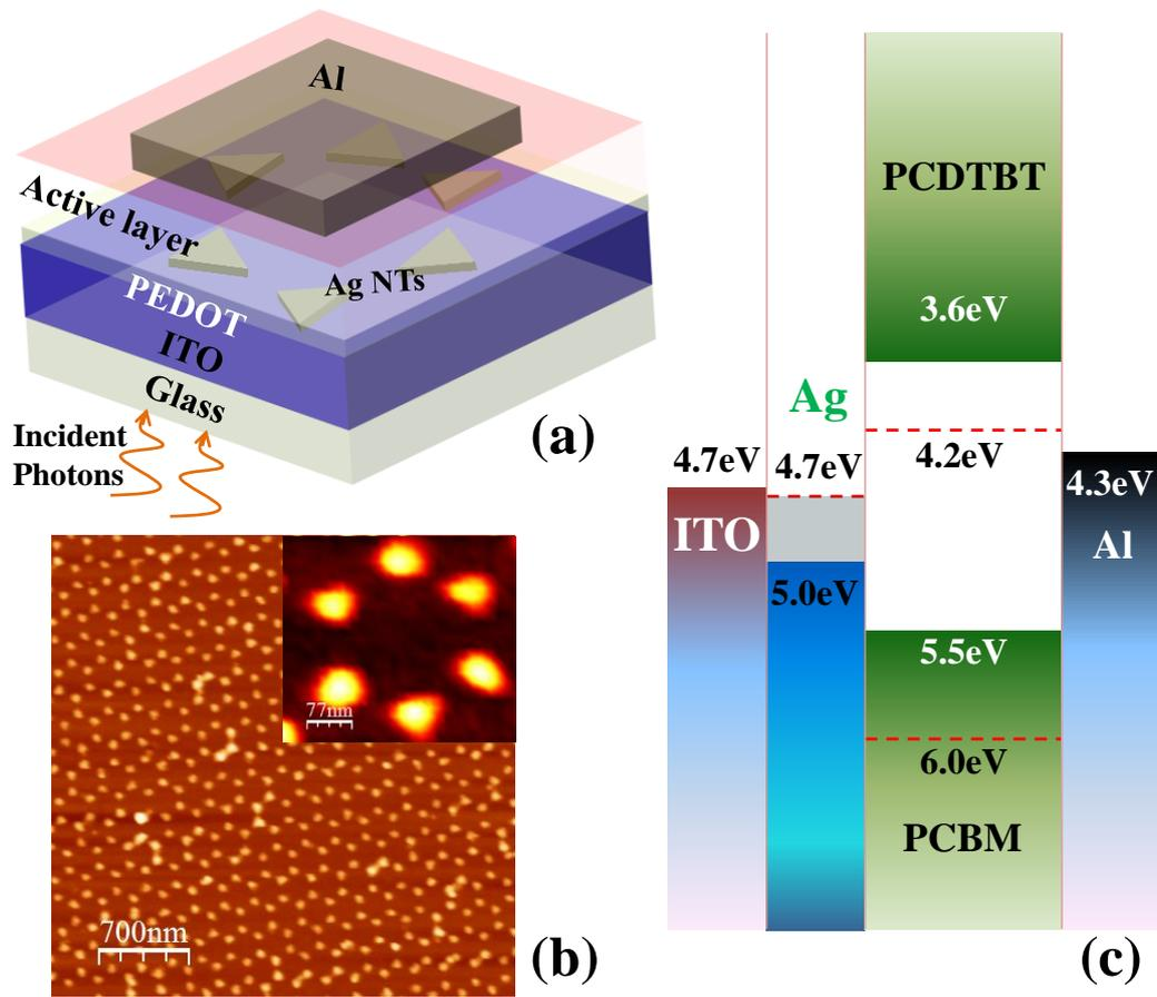
Fig1. (a) A schematic of the plasmonic organic photovoltaic device configuration investigated in our study. (b) AFM images of Ag-NT arrays. The height and side of the Ag triangles is  $\sim 20$  nm and  $\sim 40$  nm, respectively. Inset is a zoom-in of a representative unit of Ag-NT hexagonal array. (c) A schematic of the energy band alignment of the device.
