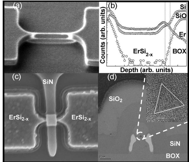
Fig. 1. (a) Tilted view SEM of two SiNWs immediately after the dry oxidation without gate oxide and silicon nitride dummy gate. The  $L_{ch}$  is approximately 500 nm. (b) SIMS depth profile of the S/D pad. (c) SEM micrograph of a completed  $\text{ErSi}_{2-x}$  N-SSDNW MOS with  $L_{ch} = 300$  nm. (d) Cross-sectional TEM of the SiNW channel showing a 8-nm-wide nanowire.
