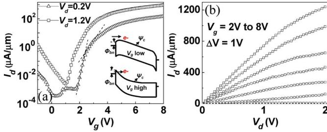
Fig. 2. (a)  $I_d$ - $V_g$  and (b)  $I_d$ - $V_d$  characteristics of an  $\text{ErSi}_{2-x}$  N-SSDNW MOS with  $L_{\text{ch}} = 500$  nm. The dashed lines in (a) clearly shows the sequential SS. The inset of (a) shows the band diagram for both low and high positive  $V_g$ s. The current was normalized by using the width of the SiNW channel.
