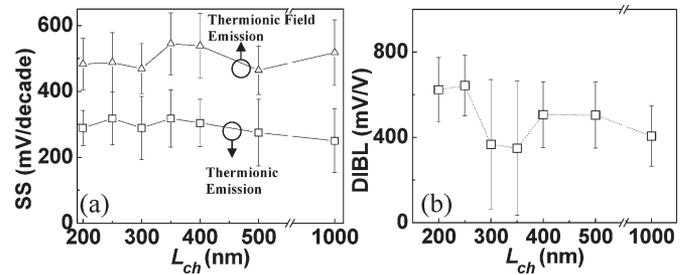
Fig. 3. Extracted transistor characteristics from  $I_d$ - $V_g$  of the  $\text{ErSi}_{2-x}$  N-SSDNW MOSs. (a) SS extracted from thermionic emission region ( $\square$ ) and SS extracted from thermionic-field emission region ( $\triangle$ ) against  $L_{\text{ch}}$  measured at  $V_d = 0.2$  V and (b) DIBL against  $L_{\text{ch}}$ .
