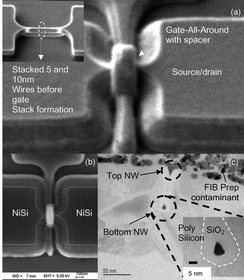
Fig. 1. (a) Tilted-view SEM of a GAA NiSi SBNWFET with  $L_g = 120$  nm before silicidation. The inset shows the tilted-view SEM of a twin-SiNW channel device after oxidation (top, 8 nm; bottom, 5 nm). (b) Top-view SEM of a device with  $L_g = 105$  nm after Ni-silicidation. (c) XTEM of the SiNW device in (b), which shows the stacked twin SiNWs. The inset shows a high-magnification XTEM micrograph of the bottom SiNW.
