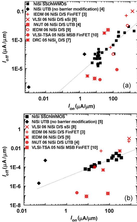
Fig. 3.  $I_{on}/I_{off}$  characteristics of the GAA NiSi (a) N-SBNWFET and (b) P-SBNWFET extracted from the  $L_g = 105\text{--}85$  nm devices.  $I_{off}$  was measured at  $V_t \pm 0.6$  V, whereas  $I_{on}$  was measured at  $V_t \pm 0.6$  V, for  $V_d = \pm 50$  mV and  $\pm 1/\pm 1.2$  V.
