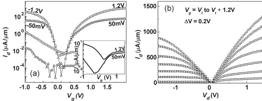
Fig. 2. (a)  $I_d-V_g$  and (b)  $I_d-V_d$  of a GAA NiSi complementary SBNWFET with  $L_g = 90$  nm. The inset of (a) shows the  $I_d-V_g$  of a GAA NiSi N-SBNWFET without S/D implantation.
