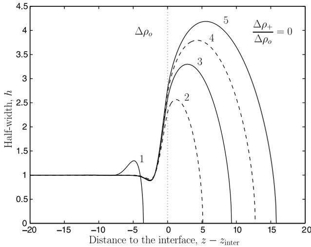
**Figure 6.** Shape of a dike that penetrates into a layer with neutral buoyancy ( $\Delta t_{1-2} = \Delta t_{2-3} = \Delta t_{3-4} = \Delta t_{4-5} = 14.364$ ). The base of this layer is at  $z = z_{\text{inter}}$  (vertical dotted line). Magma pressure profiles for times (1) and (5) are given in Figure 7 below. Note that the dike inflates above the interface and that it penetrates over large vertical distances above the interface. Calculations are made for  $K_d/K^* = 1$ .
