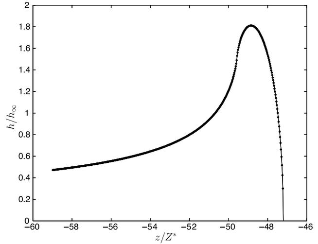
**Figure B1.** Fracture width as a function of distance in dimensionless values for a unit pressure applied over distance  $\lambda = 2.36$  at the fracture tip (see equation (B6)). Solid curve: theoretical curve (equation (B8)). Dots: calculated values over a discrete grid using the matrix formulation of the elastic problem (equation (B5)).
