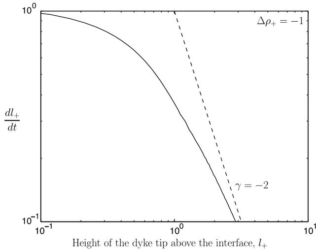
**Figure 13.** Velocity of a dike penetrating into a layer with negative buoyancy, as a function of distance above the interface. Dashed line: prediction of a simple hydrostatic model for the nose region (equation (33)).
