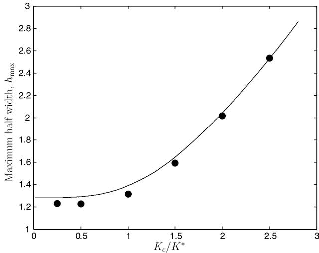
**Figure C3.** Maximum dike width as a function of dimensionless stress intensity factor  $K_c/K^*$  for steady state dikes fed at a constant rate. Solid curve: analytical results of Lister [1990]. Dots: numerical results for  $\Delta z = 2.36 \times 10^{-2}$ . The difference between numerical and analytical results is less than 4% everywhere.
