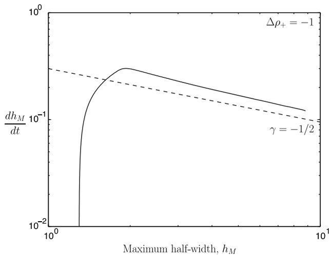
**Figure 14.** Time rate of change for the maximum dike width, as a function of maximum dike width for a dike penetrating into a layer with negative buoyancy. Dashed line: prediction of a simple hydrostatic model for the nose region (equation (34)).
