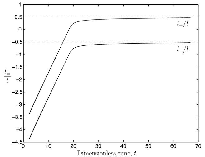
**Figure 12.** Vertical extents of the upper and lower parts of the head region of a dike that penetrates into a layer with negative buoyancy, as a function of time (in dimensionless values). For these calculations, buoyancy changes sign at the interface, such that  $\Delta\rho_+ = -\Delta\rho_o$ . Both lengths tend to the limit values predicted by a simple local hydrostatic balance (equations (28) and (29)).
