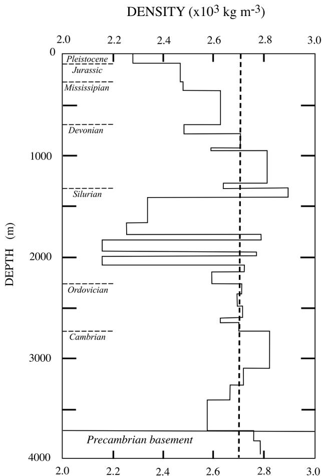
**Figure 1.** Vertical distribution of density through the sedimentary rocks of the Michigan basin from *Hinze et al.* [1978]. The vertical dashed line corresponds to the density of a typical basaltic melt.
