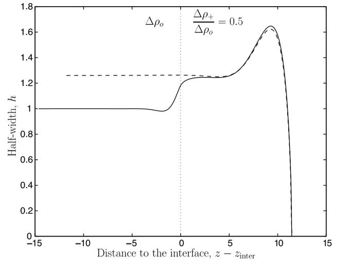
**Figure 4.** The shape of a dike that has penetrated in an upper layer of reduced buoyancy (in dimensionless values). The base of this layer is at  $z = z_{\text{inter}}$  (vertical dotted line). The dashed curve shows the steady state shape of a dike that propagates through an infinite medium with the density of the upper layer.
