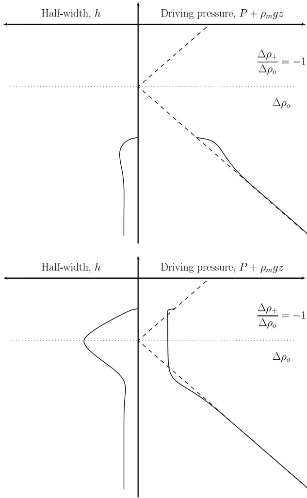
**Figure 11.** Half-width and driving pressure for a dike penetrating into an upper layer with negative buoyancy. Conventions are as in Figure 7. (top and bottom) The dike at time (1) and (2) of Figure 10. Note that the driving pressure is approximately constant in the inflated nose region when the dike has gone through the interface due to small viscous head loss.
