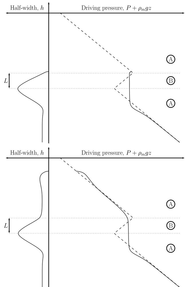
**Figure 17.** Width and driving pressure distribution in a dike that goes through a horizon with negative buoyancy (layer B,  $L = 2.840$ ). Conventions are as in Figure 7. The upper and lower panels correspond to times (2) and (4) in Figure 15. Note that the driving pressure is almost constant within the swollen dike section that develops in the negative buoyancy horizon.
