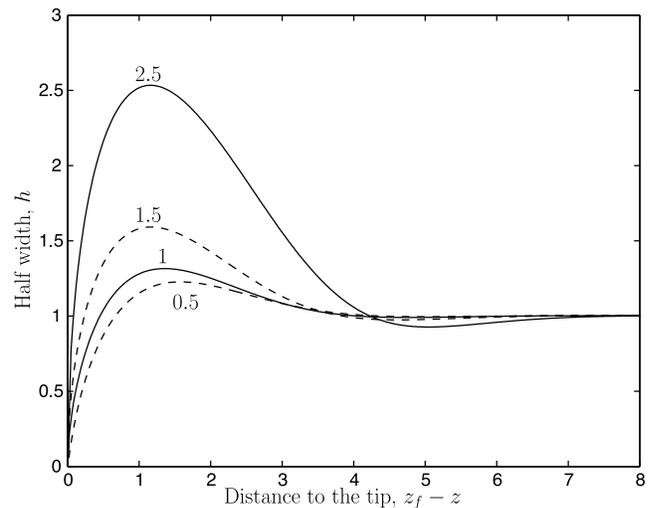
**Figure C2.** Calculated dimensionless steady state dike shapes for a fixed flux and different values of dimensionless stress intensity factor  $K_c/K^*$ , whose values are given along the curves. Results were obtained for  $\Delta z = 2.36 \times 10^{-2}$ .
