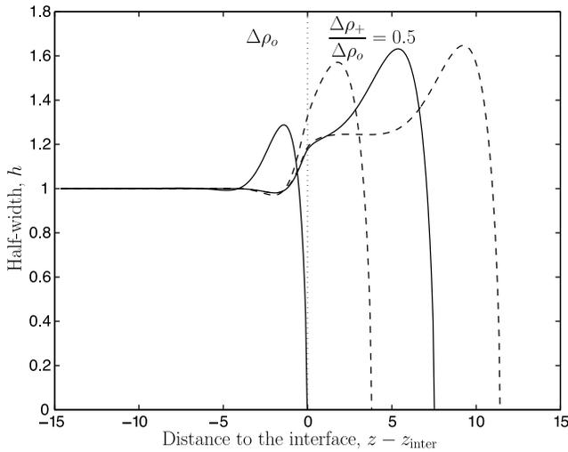
**Figure 3.** The shape of a dike penetrating into a layer with reduced buoyancy. The interface lies at  $z = z_{\text{inter}}$  (vertical dotted line). Results are shown at a fixed time interval  $\Delta t = 4.79$ . Note that the nose region rapidly adjusts to new dimensions in the upper layer. (Calculations are made for a dimensionless stress-intensity factor equal to 1, i.e.,  $K_c/K^* = 1$ ).
