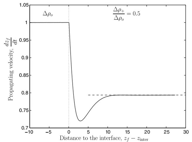
**Figure 5.** Changes of ascent velocity as a dike penetrates into a layer with reduced buoyancy. The base of this layer is at  $z = z_{\text{inter}}$  (vertical dotted line). The dashed line shows the steady state velocity in the upper layer. Note that the velocity adjustment phase is spread over a large vertical distance above the interface.
