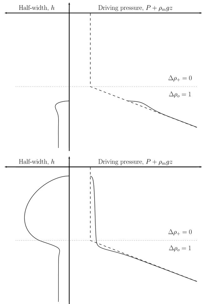
**Figure 7.** Half-width  $h$  and driving pressure  $P_d$  for a dike penetrating in a medium with neutral buoyancy at times (1) and (5) of Figure 6. Driving pressure is that which determines the flow rate and is defined by equation (7). Here it is shown to within an arbitrary constant. The dashed line is such that  $\partial P_d / \partial z = -\Delta\rho g$ , where  $\Delta\rho = \rho_s - \rho_m$ , corresponding to zero internal overpressure within the dike.
