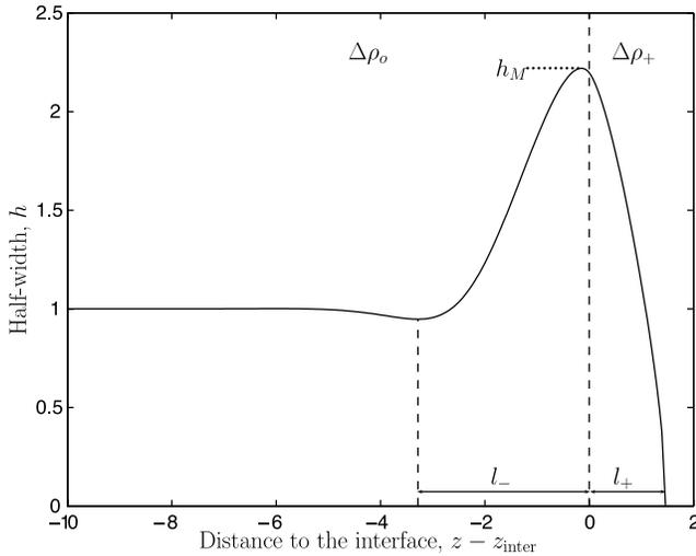
**Figure 2.** Definition of the characteristics of a dike going through a density interface located at  $z = z_{\text{inter}}$ .  $l_+$  and  $l_-$  stand for the lengths of the nose region above and below the interface, respectively. Total nose length is  $l = l_- + l_+$ , and nose width is  $h_M$ . For typical geological values, a dimensionless half-width of one corresponds to 1 m and a dimensionless distance of one corresponds to 1 km (see text for details).
