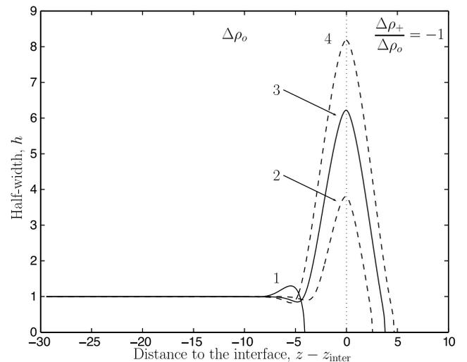
**Figure 10.** A dike penetrating into a layer with negative buoyancy ( $\Delta t_{1-2} = \Delta t_{2-3} = \Delta t_{3-4} = 14.364$ ). The distributions of driving pressure at times (1) and (2) are given in Figure 11. Note that the dike is able to overshoot the interface and that it swells markedly. ( $K_c/K^* = 1$ ).
