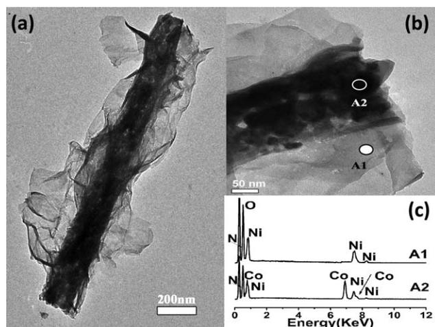
**Fig. 2** TEM images of an individual hybrid nanostructure. The EDS signals of the areas labeled as A1 and A2 in (b) are shown in (c).
