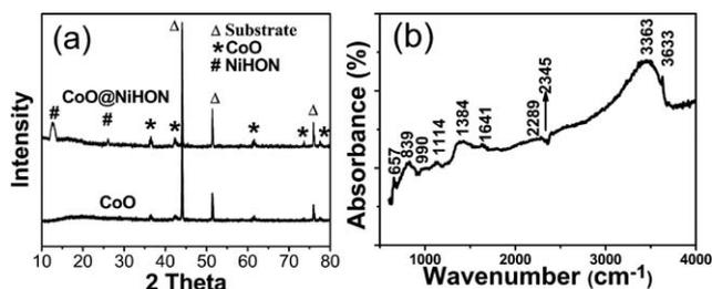
**Fig. 3** (a) XRD patterns of the CoO nanowire and the hybrid structure on the nickel foam. (b) FTIR spectrum of the hybrid structure.
