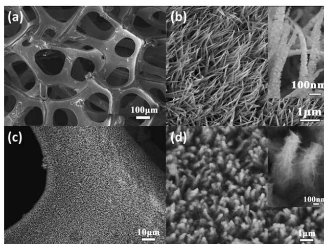
**Fig. 1** SEM images of (a) the 3D structure of nickel foam, (b) the CoO nanowire on the nickel foam. (c,d) low and high magnification images of the hybrid structure on the nickel foam. Insets in Fig. 1b and 1d are the enlarged pictures.
