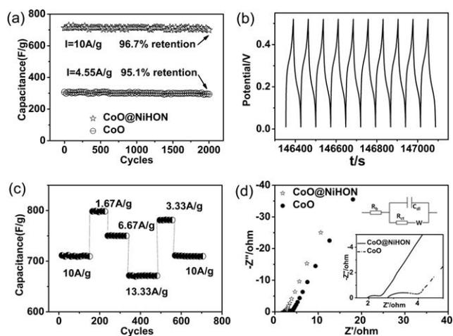
**Fig. 5** (a) Cycling performance of the hybrid structure and CoO nanowires. (b) Last 10 charge–discharge curves of the hybrid structure. (c) The current density dependence of the hybrid structure. (d) Impedance Nyquist plots of the hybrid structure and CoO nanowires on nickel foam at open circuit potential.
