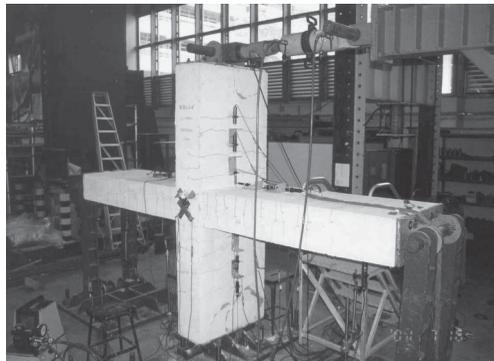
**FIGURE 2** Test setup showing Specimen IWB2.
