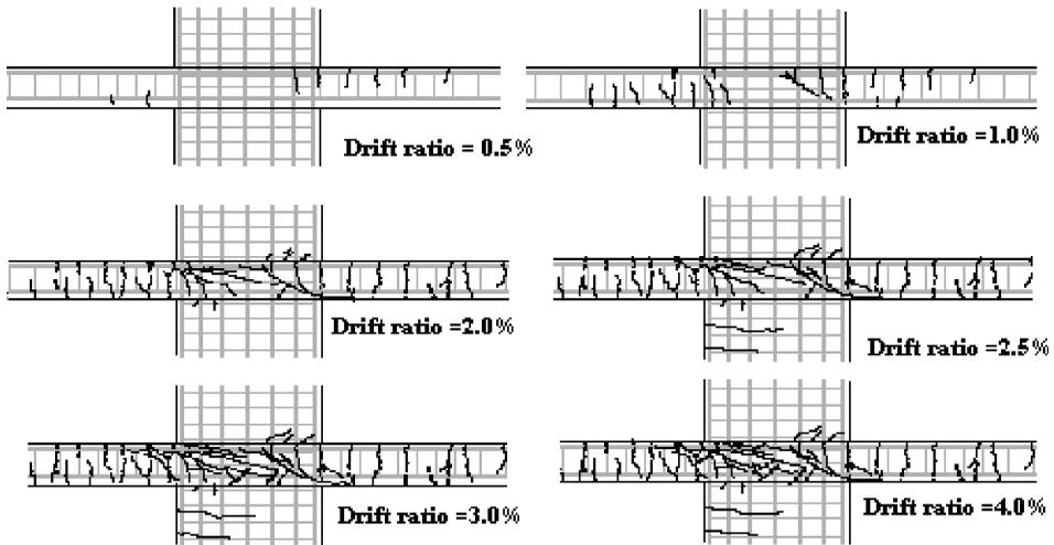
FIGURE 7 Cracking pattern of Specimen IWB3.
