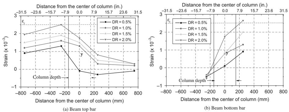
FIGURE 12 Strain profiles of beam reinforcement, Specimen IWB2.
