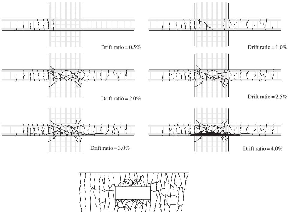
**FIGURE 6** Cracking pattern of Specimen IWB1.
