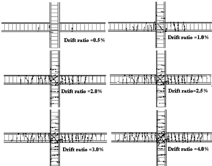
FIGURE 11 Cracking pattern of Specimen IWB2.
