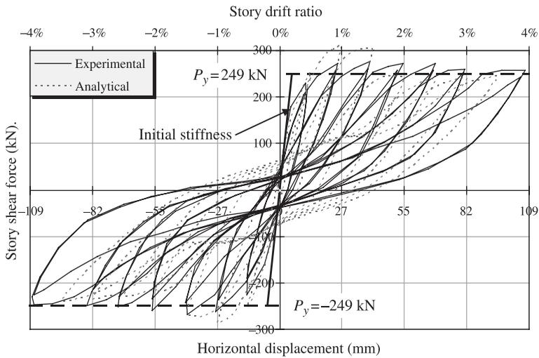
**FIGURE 4** Comparison of hysteresis loops between the experimental tests and those predicted by numerical analysis for Specimen IWB1.
