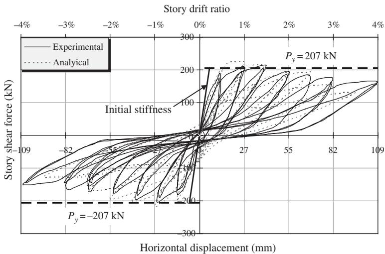
**FIGURE 10** Comparison of hysteresis loops between the experimental tests and those predicted by numerical analysis for Specimen IWB2.
