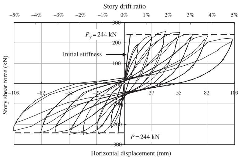
**FIGURE 5** Hysteresis loops showing story shear force versus horizontal displacement for Specimen IWB3.
