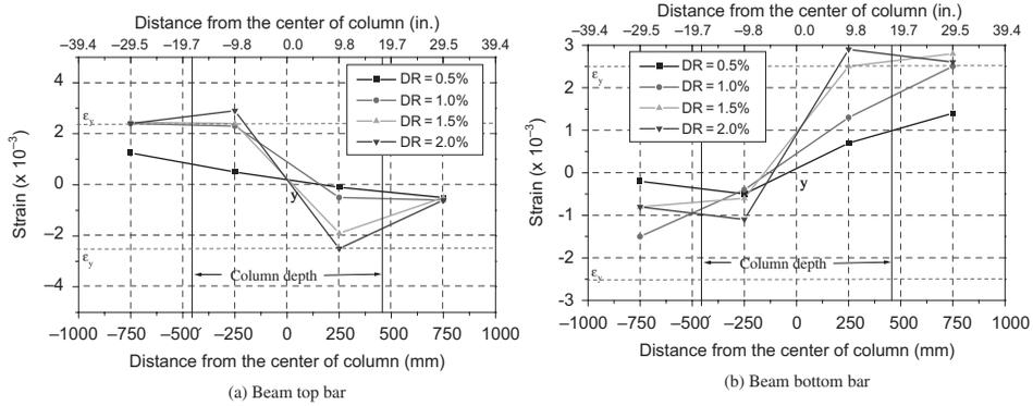
**FIGURE 9** Strain profiles of beam reinforcement, Specimen IWB3.
