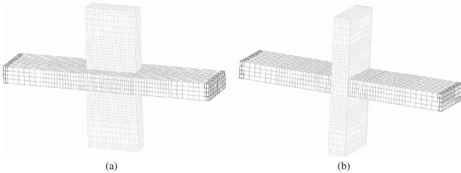
**FIGURE 14** Finite element modeling of the specimens (a) Specimen IWB1; (b) Specimen IWB2.
