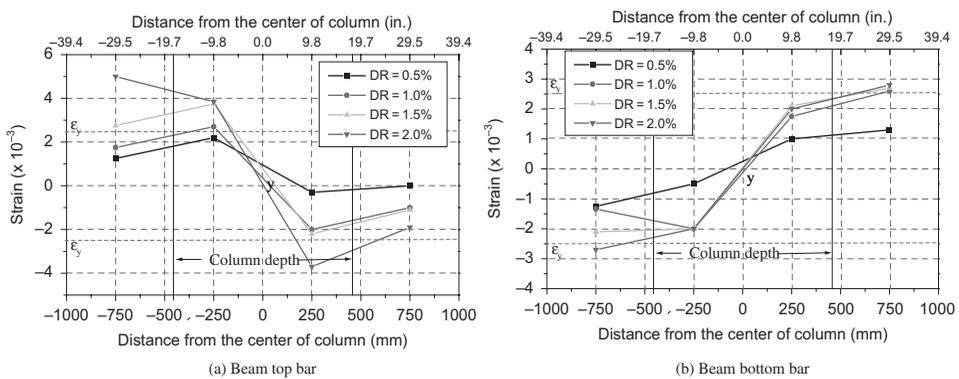
FIGURE 8 Strain profiles of beam reinforcement, Specimen IWB1.
