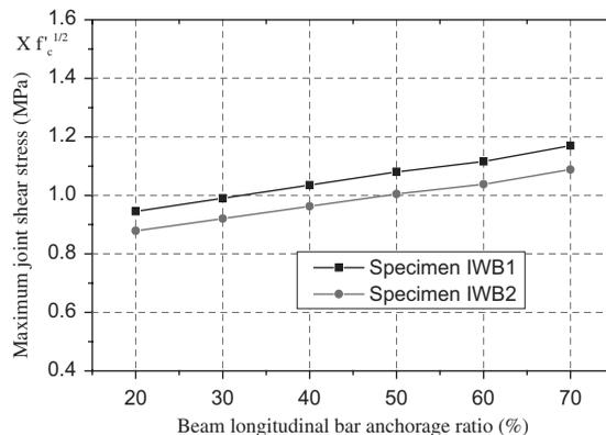
FIGURE 17 Influence of beam longitudinal bars anchorage on joint shear stress.
