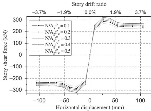
**FIGURE 15** Influence of axial load variation on the story shear forces predicted by FE analysis, Specimen IWB1.
