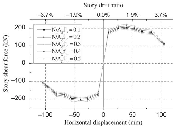
**FIGURE 16** Influence of axial load variation on the story shear forces predicted by FE analysis, Specimen IWB2.
