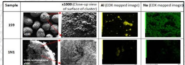
Figure 1 Structural characterization of spherical clusters by SEM-EDX
