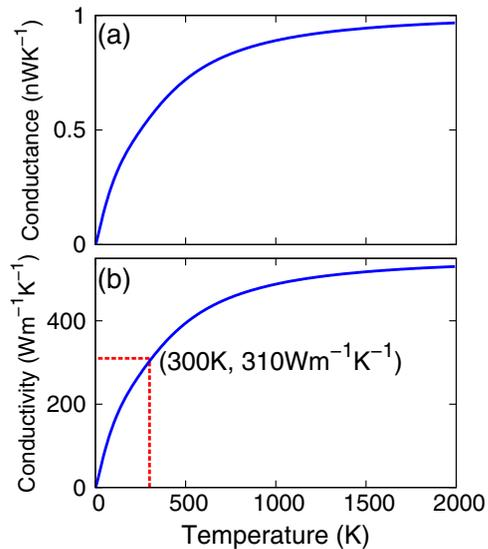
FIG. 3. Thermal transport properties in the polyethylene chain. (a) Thermal conductance versus temperature. (b) Thermal conductivity ( $\kappa$ ) calculated from thermal conductance ( $\sigma$ ) by  $\kappa = \sigma L/s$ , with cross-sectional area  $s = 18.24 \text{ \AA}$ . The length  $L = 100 \text{ nm}$ .
