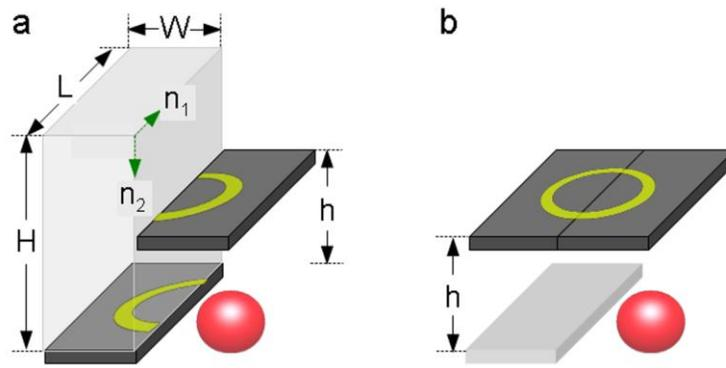
Fig. 1. (a) A cuboidal phase-preserved optical elevator is made of a single piece of natural birefringent crystal with the geometrical parameters of  $H = 19.8\text{mm}$ ,  $L = 40\text{mm}$ , and  $W = 10\text{mm}$ . (b) The phase-preserved elevating design virtually lifts a sheet to a height of  $h = 2.2\text{mm}$ , enlarges the volumetric space under the sheet, and further provides the camouflage capability of exterior environment.
