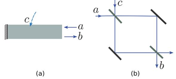
FIG. 3. (Color online) (a) Schematic of a one-channel absorbing cavity, where the output amplitude  $b$  is a superposition of the input amplitude  $a$  and the reservoir operator  $c$ . (b) The corresponding Mach-Zehnder interferometer, with  $a$  and  $c$  entering in the two input ports and  $b$  being one of the outputs.
