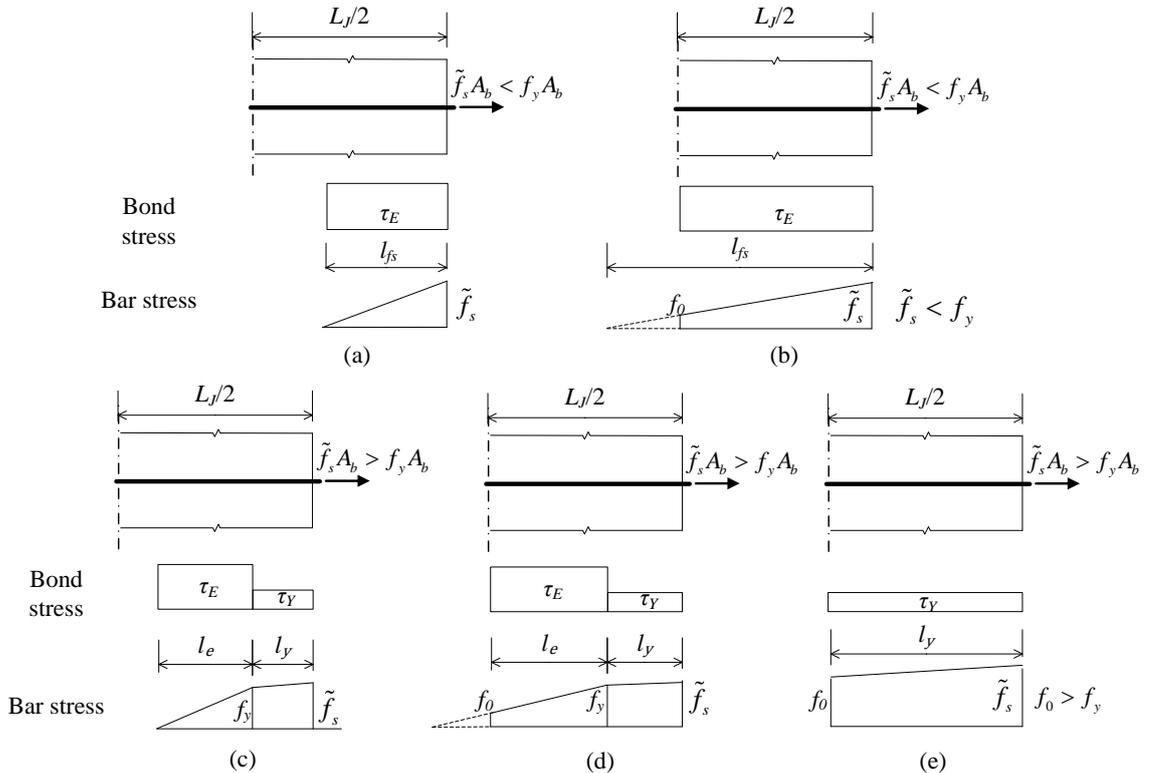
Fig. 3 Stress propagation of the steel reinforcement and the corresponding bond stress
