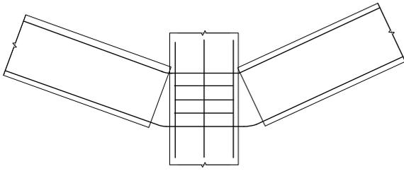
Fig. 1 Additional deformation resulting from local bar slip at the “fixed end condition”
