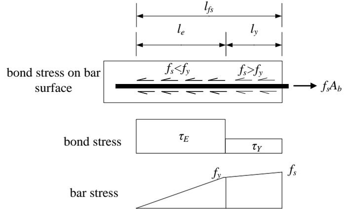
Fig. 2 Assumed bond stress and bar stress distribution for a reinforcing bar anchored in a joint
