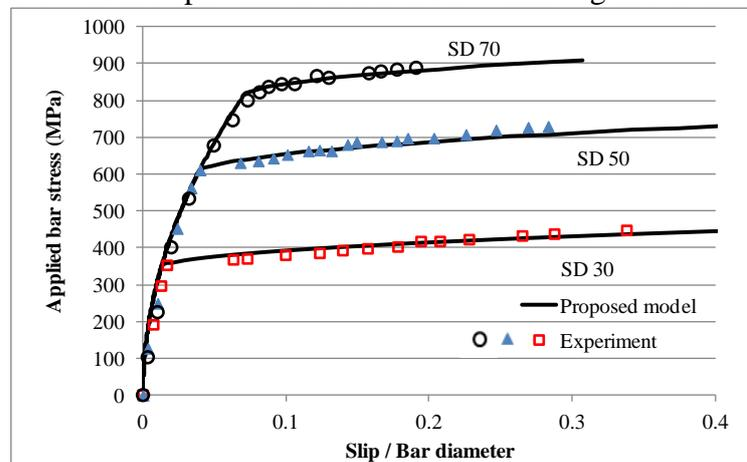
Fig. 4 Relations between the slip at the loaded end and applied bar stress in Shima's tests [4]
