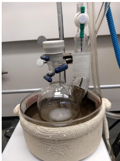
Figure 1. Reaction Setup for Step A (acetophenone oxime)
