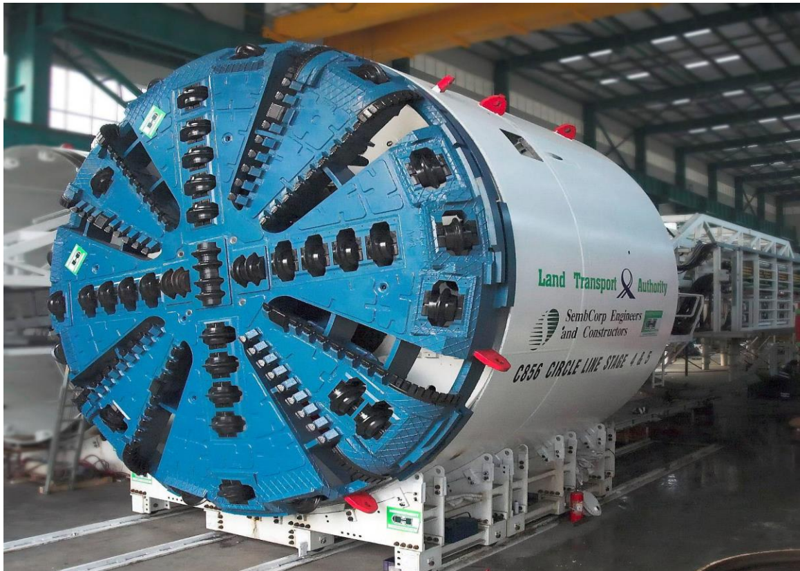
Figure 4.3 Illustration of Earth Pressure Balance Machine (EPBM)
