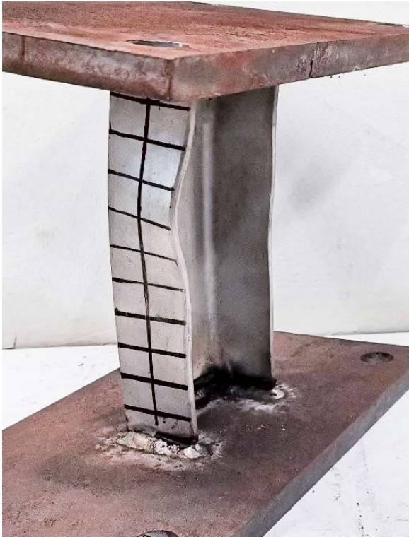
Figure 5.2. Experimental and numerical failure modes for specimen C5 failing in the 'C' orientation.
