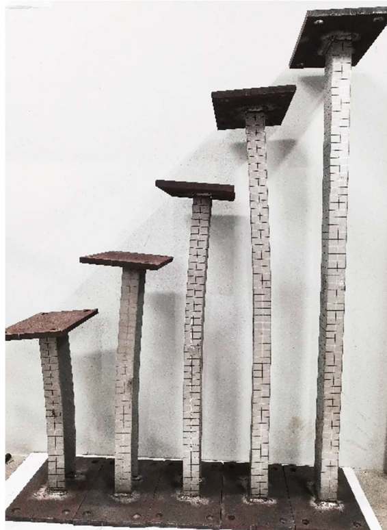
(b) C 100×50×5 specimens (from left to right: C2-L1, C2-L2, C2-L3, C2-L4 and C2-L5)
