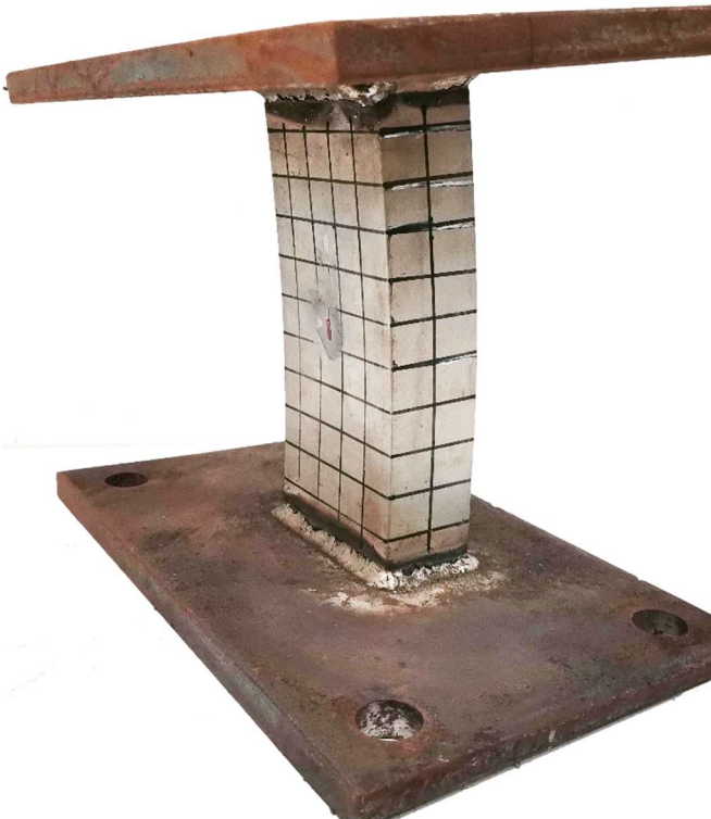
Figure 5.3. Experimental and numerical failure modes for specimen RC4 failing in the 'reverse C' orientation.
