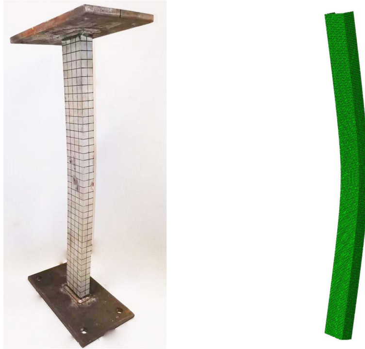
Figure 7.2. Test and FE failure modes for specimen A3 (with minor-axis global buckling in the ‘reverse C’ orientation).
