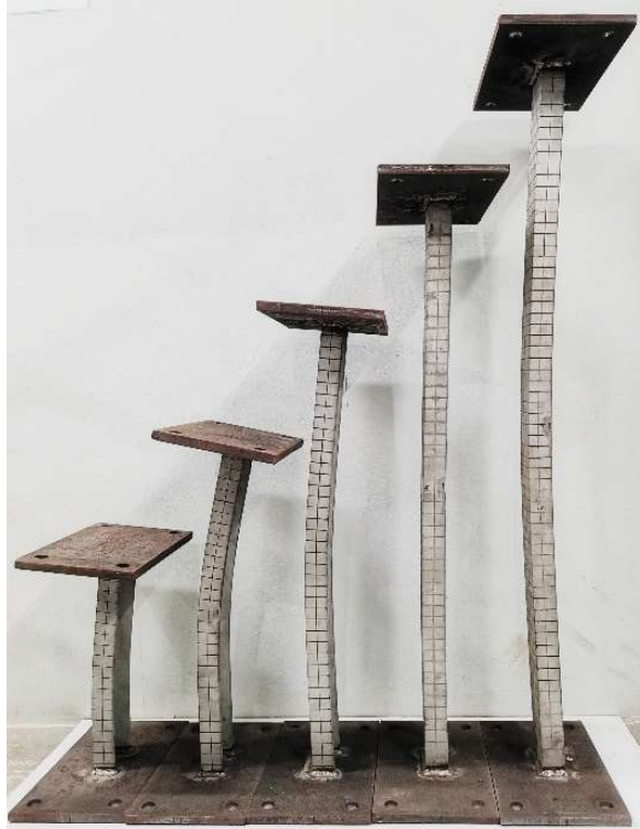
(a) C 80×40×5 specimens (from left to right: C1-L1, C1-L2, C1-L3, C1-L4 and C1-L5)
