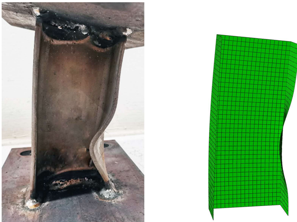
Figure 4.4. Test and FE failure modes for stub column specimen A5.
