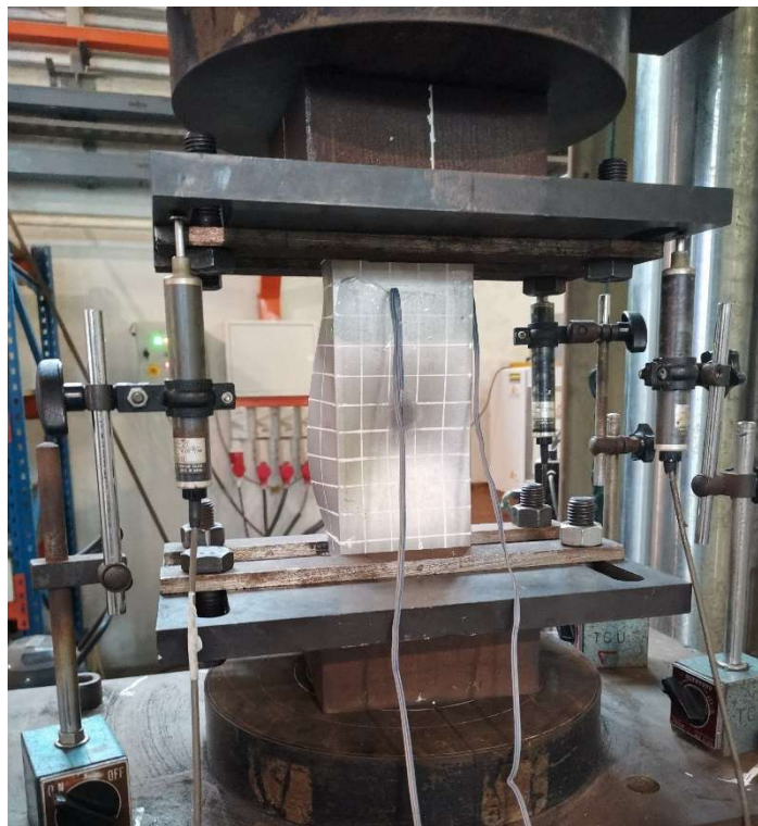
Figure 3.11. Stub column test setup.
