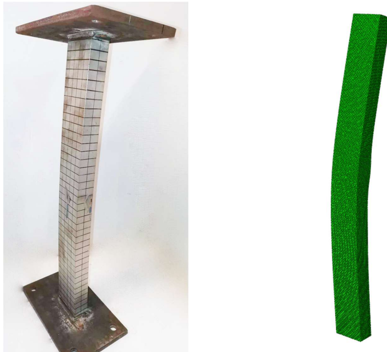
Figure 7.3. Test and FE failure modes for specimen B3 (with minor-axis global buckling in the ‘C’ orientation).
