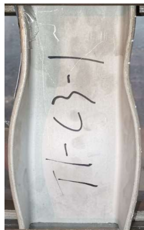
Figure 3.13. Test and FE failure modes for typical stub column specimens.
