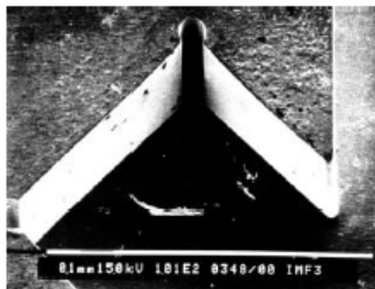
Figure 2.9 Alumina micro optical bench [2]
