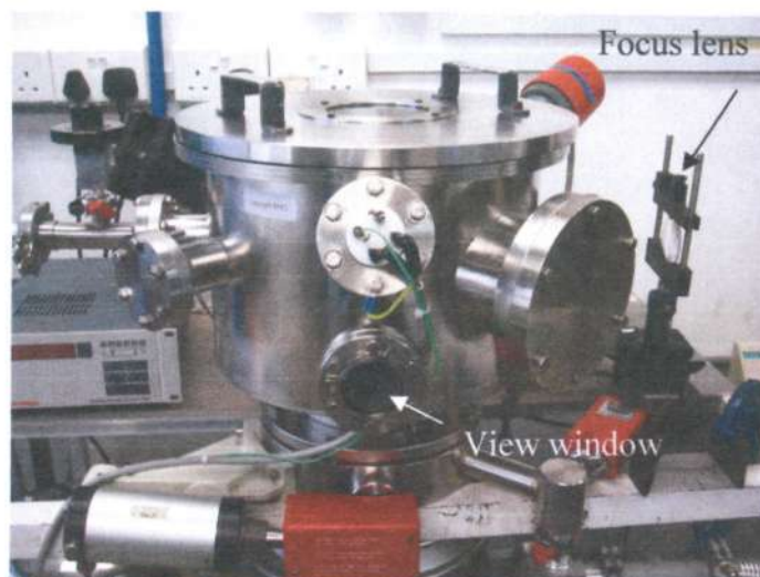
Figure 3.2 Photograph of the pulsed laser deposition chamber.
