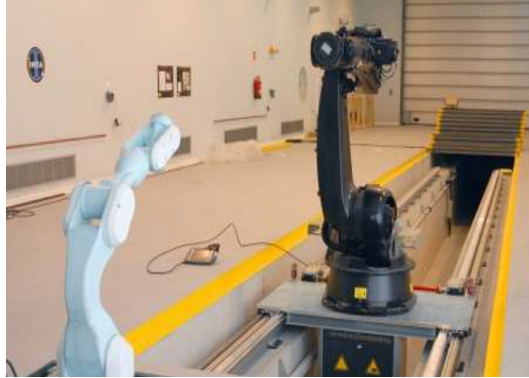
FIGURE 2.2: GMV, Spain Robotic Based Rendezvous & Docking Simulator [11]
