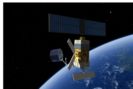
FIGURE 1.10: Robotic Capture Concept [7]
