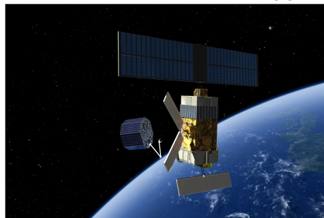
FIGURE 1.4: Autonomous - Uncooperative Target: Space Debris Capture [4]
