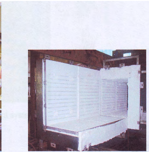
Figure 3.2 L-shaped electric furnace
