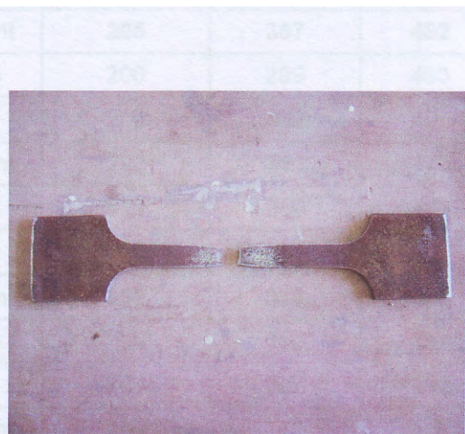
Figure 3.11 Coupon after tensile test
