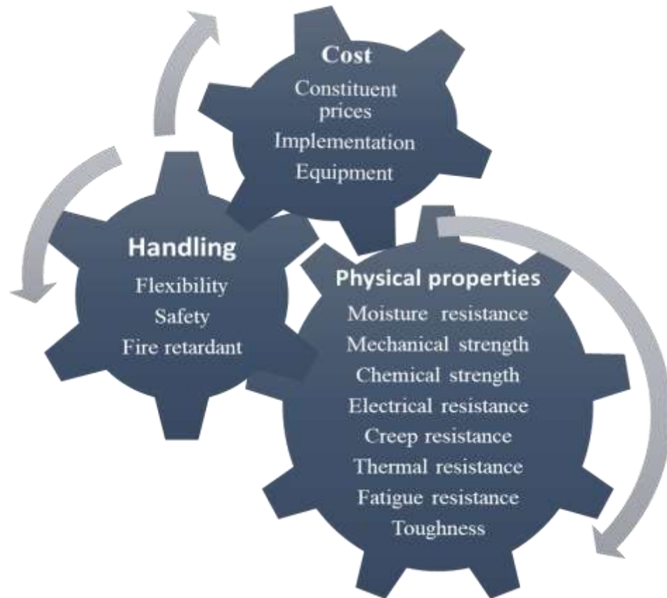
Figure 1- 2 Desired features of encapsulation material designed for HTHE operations
