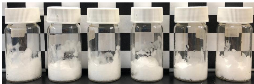
Figure A.5.3 Glass vials with the ternary DODAC-water-dimethyl urea mixtures. Increasing additive concentration from left to right (5.0, 7.5, 10.0, 12.5, 15.0 and 20.0 wt. %).
