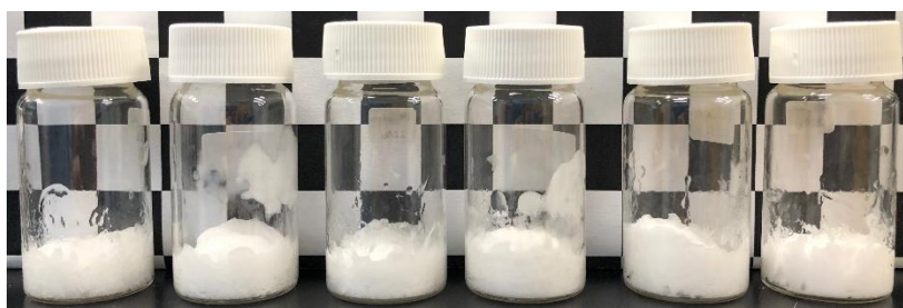
Figure A.5.2 Glass vials with the ternary DODAC-water-methyl urea mixtures. Increasing additive concentration from left to right (5.0, 7.5, 10.0, 12.5, 15.0 and 20.0 wt. %).
