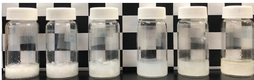
Figure A.5.8 Glass vials with the ternary DODAC-water-hexanoic acid mixtures. Increasing additive concentration from left to right (5.0, 7.5, 10.0, 12.5, 15.0 and 20.0 wt. %).
