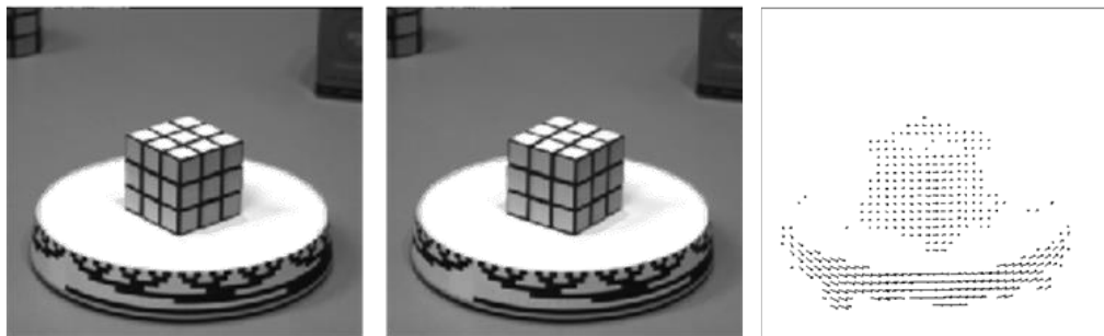
Figure 2.26 An example optical flow field in vector expression of a rotating object.
