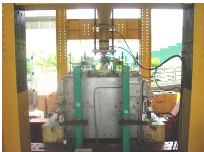
Figure 5.1 Unrestrained Shear Component Test Set-up
