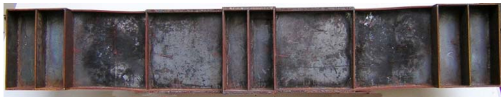
(c) Deformed shape for RTG4-3 tested at 670 °C
