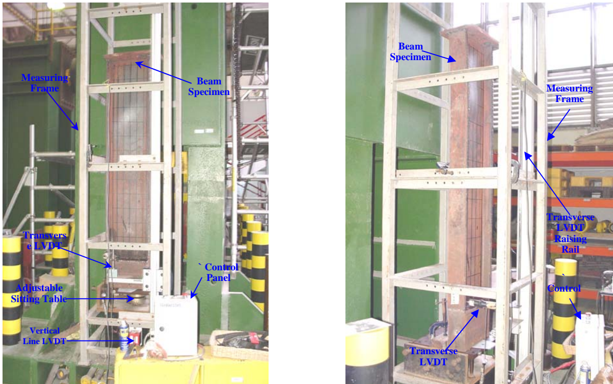
Figure 7.13 Measurement Scanning System Details
