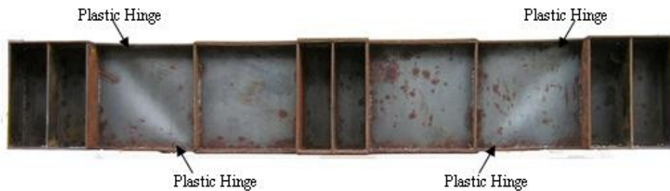
(a) Deformed shape for RTG4-1 tested at 400 °C
