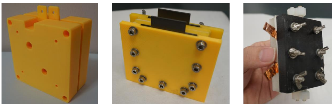
Figure 5.4. Assembled test cell prototype. (a) With flow-by configuration. (b) Type 1 flow-through configuration (c) Type 2 flow-through configuration.
