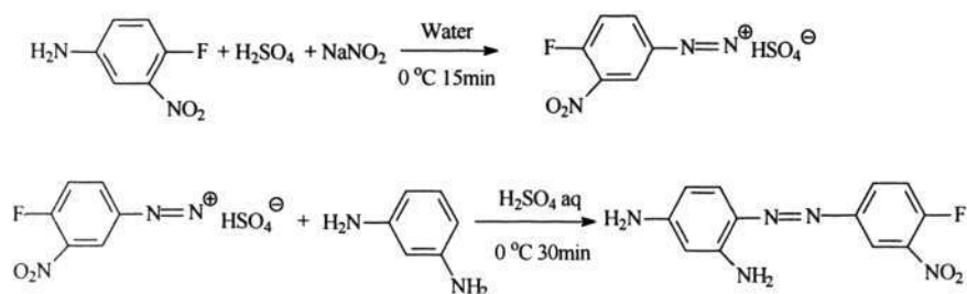
Figure 3-6 Synthetic route of 2R-4F-3N-DIAMINE
