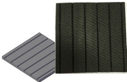
Figure 18. Flow channel design on the porous electrode.
