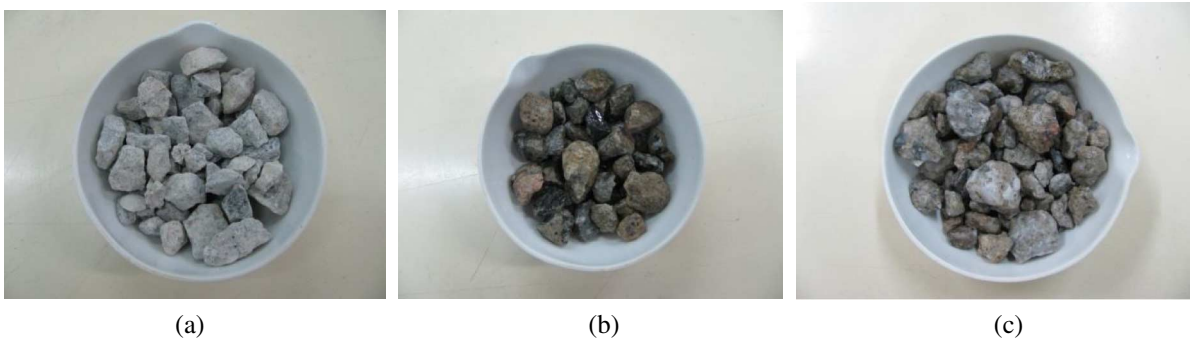
FIG. 1 Photographs of RCA: (a) RCA (Uncoated), (b) RCA (Oil), and (c) RCA (Wax).
