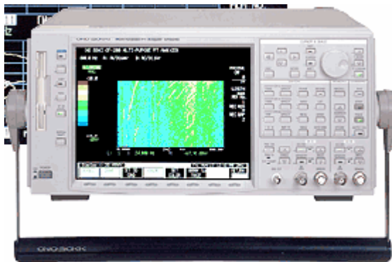
Figure 6.19 ONO SOKKI Multi-Purpose FFT analyzer (CF-5220Z).
