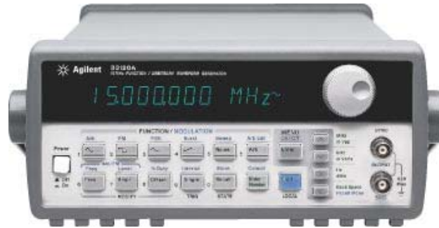
Figure 6.16 HP/Agilent 33120A Function generator.
