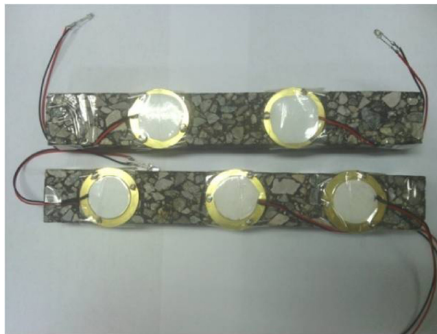
FIG. 2. Beam test piece installed with piezoelectric patches.
