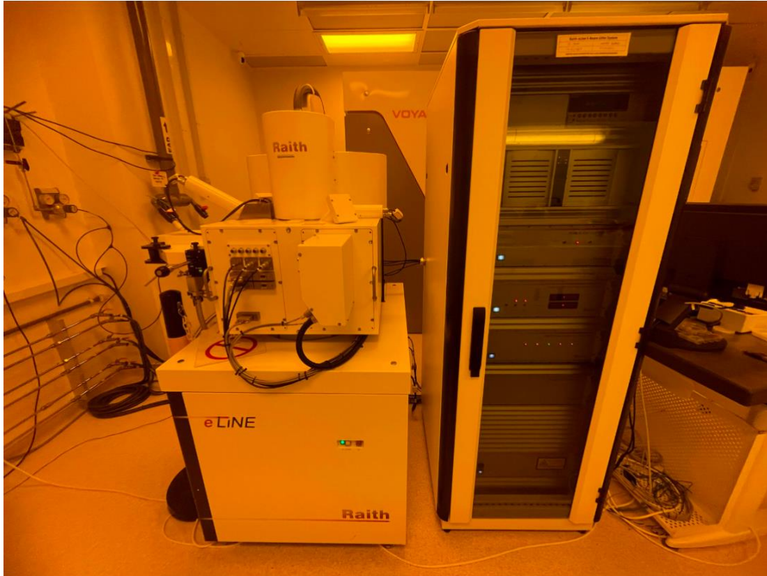
Fig. 3.2: Image of an Electron Beam Lithograph Setup (Raith eLine EBL)
