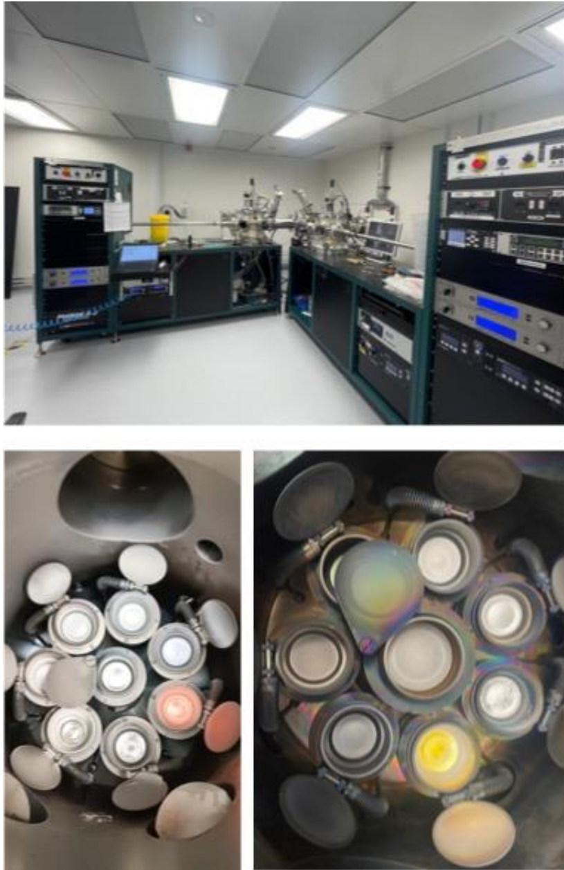
Fig. 3.1: (Top) Image of two customized-made AJA ATC-Orion 9 UHV sputtering system (Bottom) Two x 8 different targets in the main chamber
