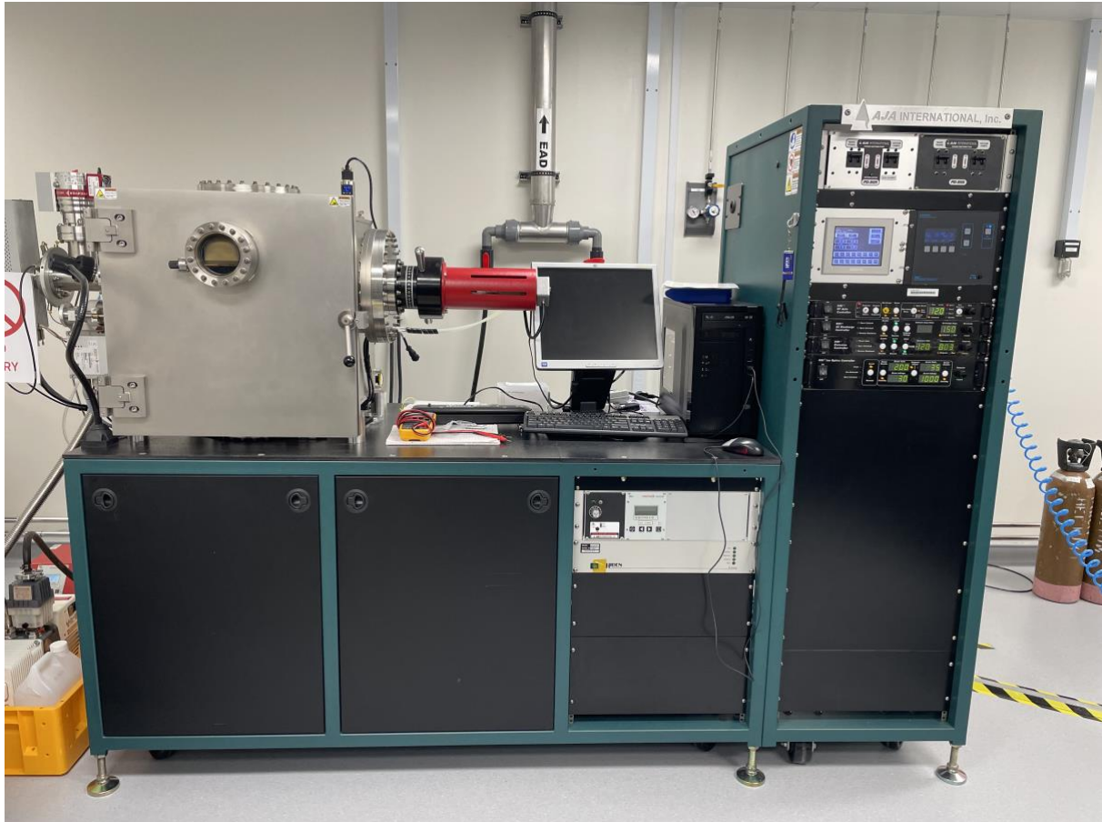
Fig. 3.4: Image of a ion-beam etching setup
