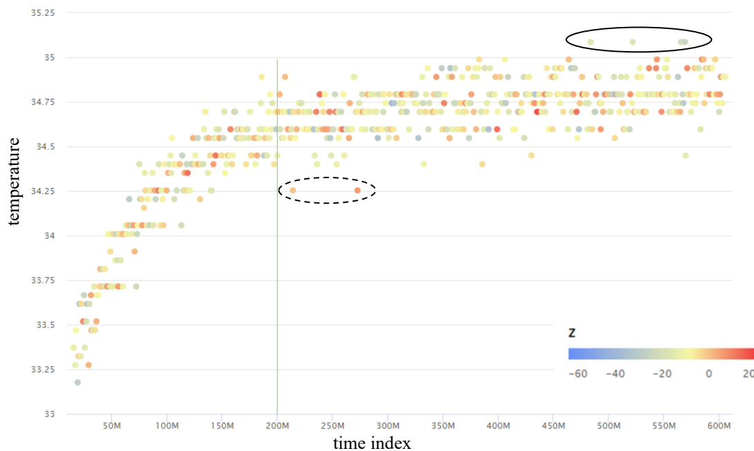
Figure 6.5: The accelerometer temperature variation during the test.
