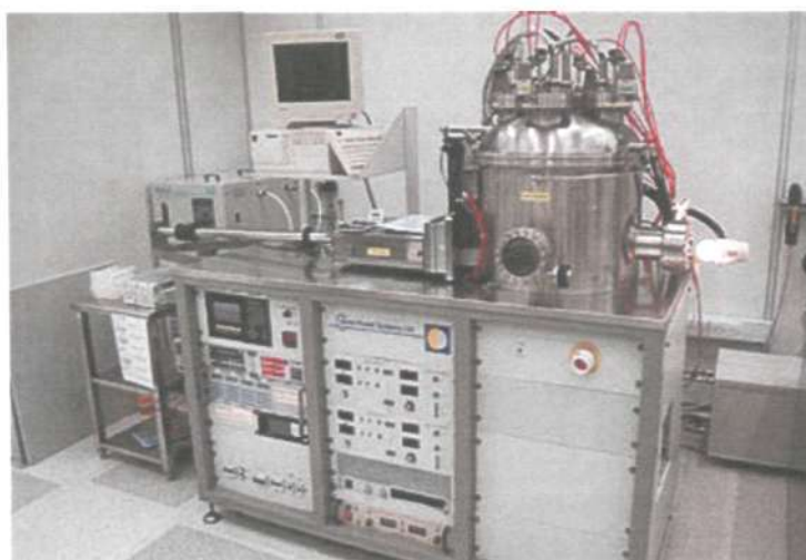
Fig B.5: Sputtering equipment
