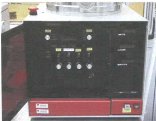
Fig B.4: Micro RIE equipment
