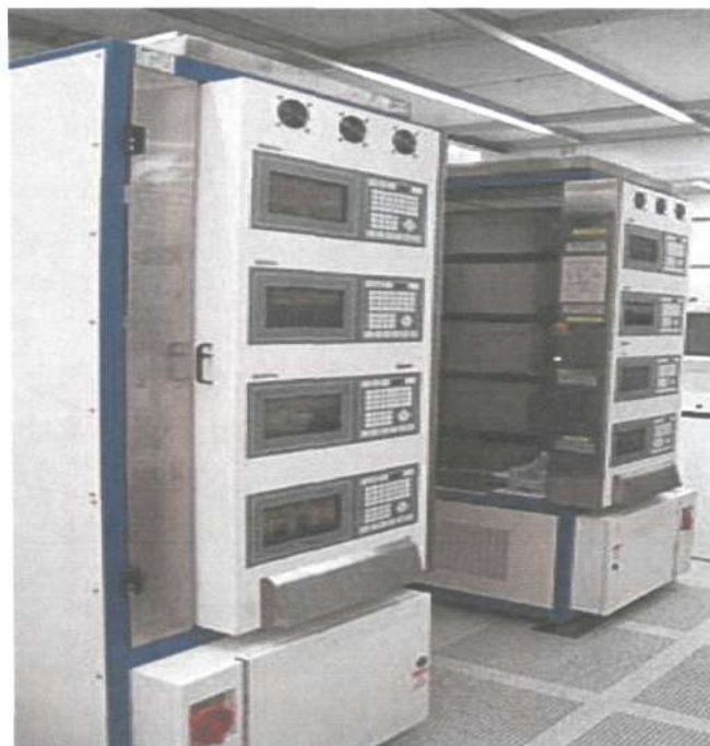
Fig B.3: Tystar furnaces for thermal oxidation and LTO
